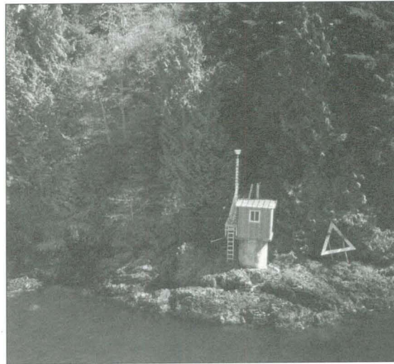
The tide station in Tofino measures water levels as part of the tsunami warning systems.
