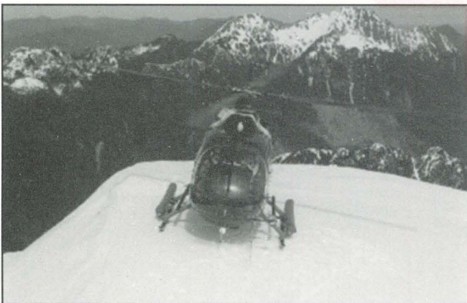
Due to the possibility of unstable snow cornices on the landing pads, all touchdowns were done "hot" with the engines under full power.
