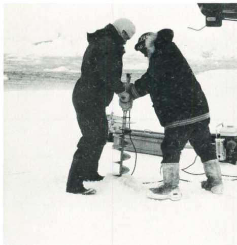
Using a portable CTD lowered through holes drilled in the ice, Ron Perkin and Oolalteetah Iqaluk, an Inuit from Grise Fjord, map the lateral distribution of warm water.
