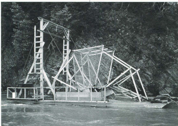
A fishwheel similar to this one on the Nass River, was used to capture steelhead and coho for radio-tagging.
