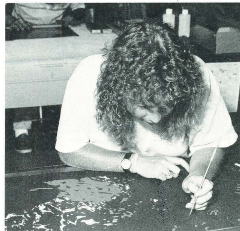
Everything must be accurate on a nautical chart and quality control is a rigorous part of each stage of the production process. A cartographer touches up a four-colour tint negative.
