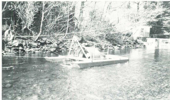
A rotary screw trap, floated on pontoons, is used to capture coho smolts in Lachmach River, one of the study areas in the Skeena Watershed. The coho are counted, measured and coded-wire tagged before being released.
