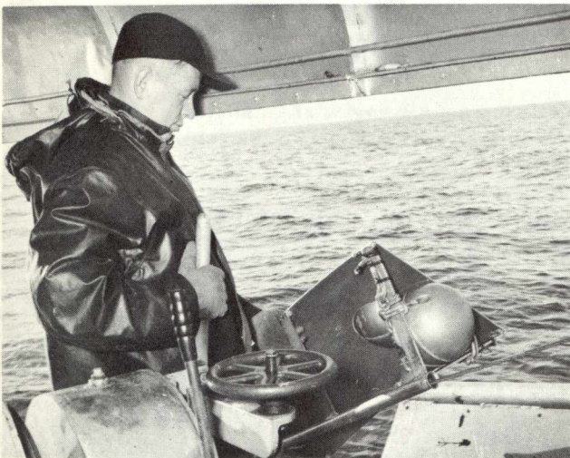
Preparing to let the hydroplane float go on the port side.
