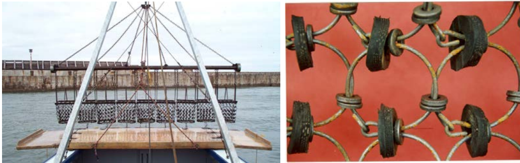
Figure 3. Digby-type drag commonly used in the commercial scallop fishery in DFO Gulf Region showing tow bar and steel ring buckets. In the panel on the right is shown the configuration of the bucket showing rings linked with steel washers and vertically placed rubber washers.
