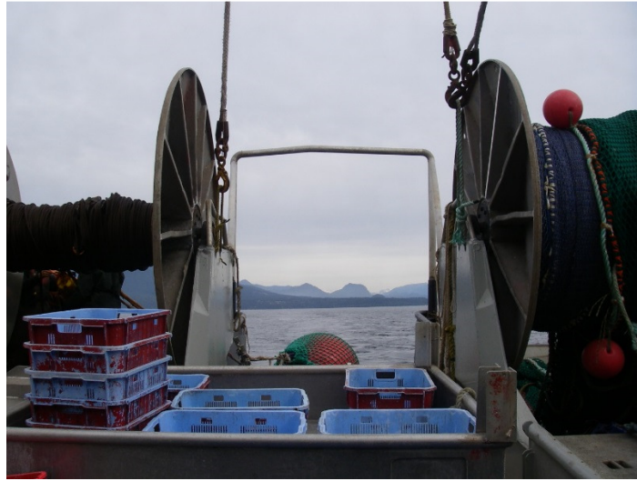
Figure 1. Back deck of the FV Sea Crest with the Cantrawl 250 net deployed off the left drum and the LFS 7742 net stored on the right drum. The large float in the centre was one of two large floats deployed on the surface tows. The blue baskets are used for sorting and weighting the biological samples. Photo by Jackie King.
