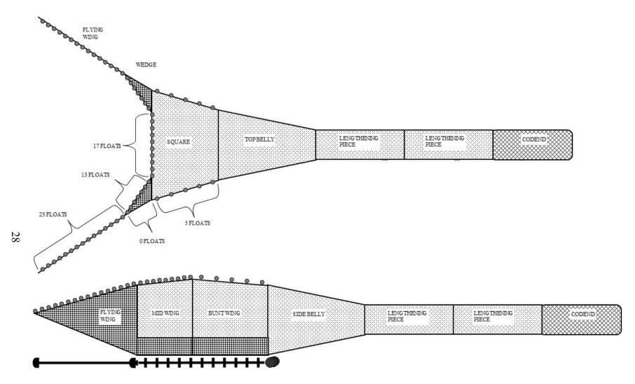
Figure 4. Top and side view of the Atlantic Western IIa box trawl used on the 2017 HS synoptic bottom trawl survey.
