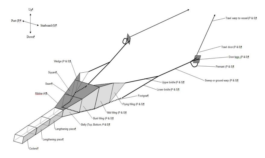
Figure 3. Overview diagram of the Atlantic Western IIa box trawl used on the 2017 HS synoptic bottom trawl survey.
