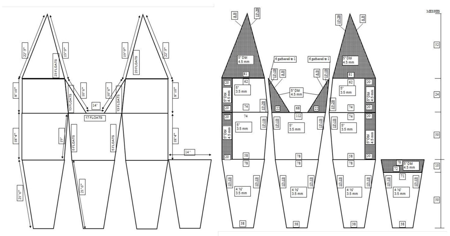
Figure 6. Details of the wing and belly sections of the Atlantic Western IIa box trawl used on the 2017 HS synoptic bottom trawl survey. Dimensions and the float arrangement are shown on the left while netting details, mesh counts, and mesh cuts are shown on the right side of the diagram.
