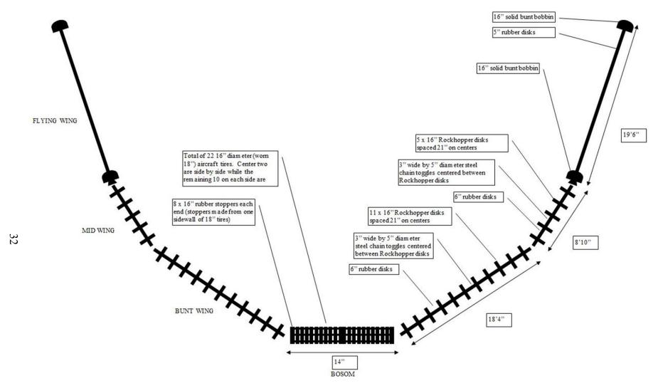
Figure 8. Details of the Rockhopper foot gear for the Atlantic Western IIa box trawl used on the 2017 HS synoptic bottom trawl survey.
