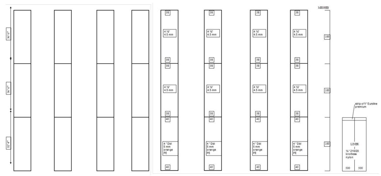
Figure 7. Details of the lengthening (intermediate) pieces and codend sections of the Atlantic Western IIa box trawl used on the 2017 HS synoptic bottom trawl survey. Dimensions are shown on the left while netting details, mesh counts, and mesh cuts including the codend liner are shown on the right side of the diagram.
