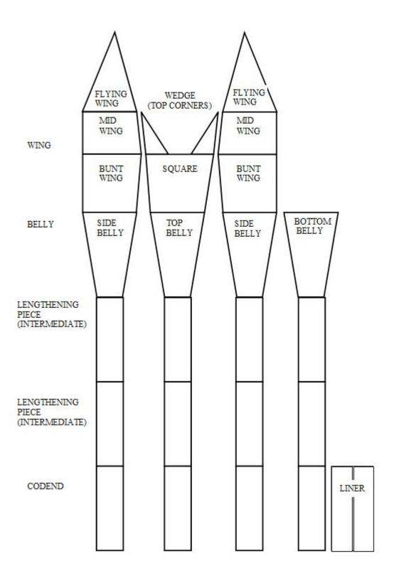
Figure 5. Diagram of the net panels with section names for the Atlantic Western IIa box trawl used on the 2017 HS synoptic bottom trawl survey.
