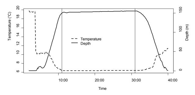
Figure 13. Example of a Seabird 39 temperature and pressure profile collected during a synoptic bottom trawl survey. The vertical lines indicate the start and end of net contact with the sea floor.
