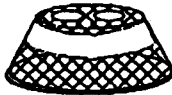
1991 - First Experiment Angle panel relocated in the upper part of the angle slope of the conical trap.
