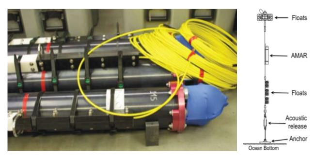
Left: Autonomous Multichannel Acoustic Recorders (AMARs) manufactured by JASCO Applied Sciences (photo: H. Moors-Murphy). Right: Sample AMAR mooring diagram.
