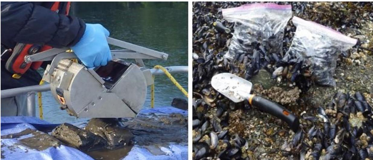
Figure 30-2. Sediment samples are collected using a petite ponar grab (left), while mussel samples are collected by hand (right).
