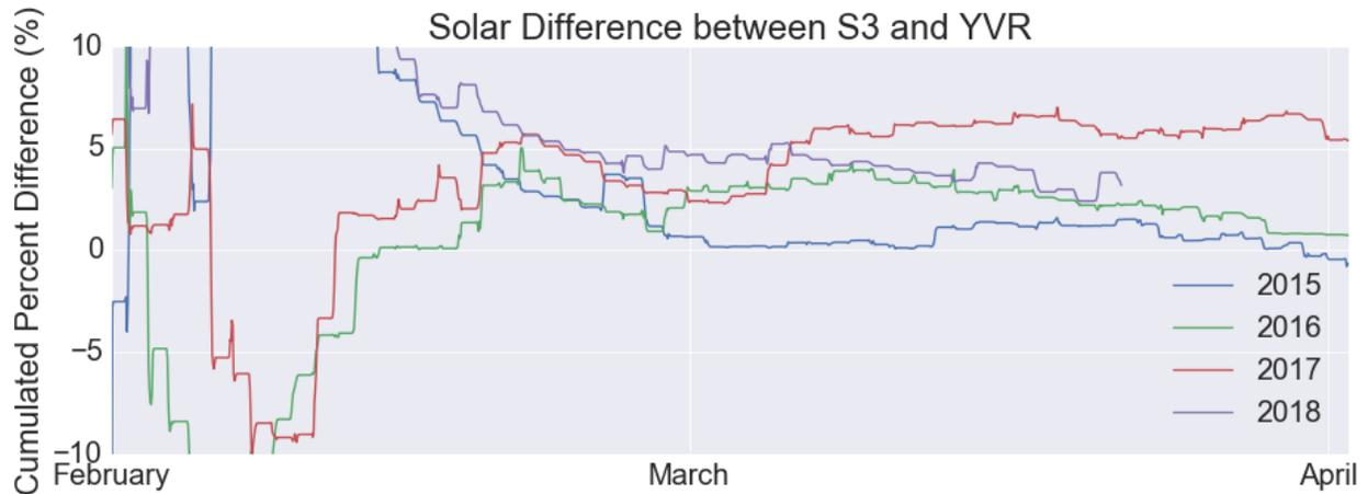
Figure 37-1. The cumulative percent difference between the solar radiation at Station S3 and at YVR airport, starting in February of each year. The solar radiation values are taken from Canada's HRDPS system (Environment Canada, 2018). In 2017, S3 was 7% brighter than YVR whereas in 2015, 2016 and 2018 the difference was less than 4%.
