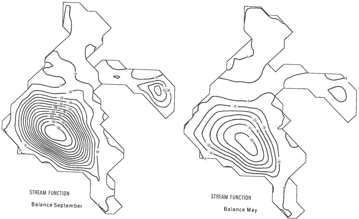
Figure 3 Stream function (for the volume transport) in units of 10^{12} \text{ cm}^3 \text{ sec}^{-1} for September (left) and May (right) using data averaged over 30 years.
