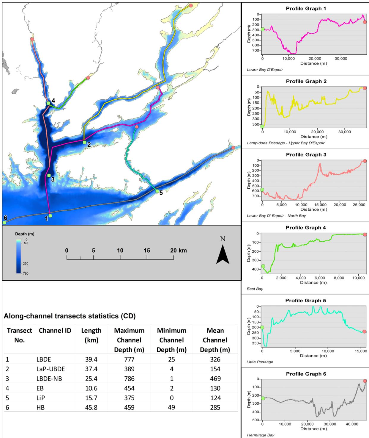
Figure D1: Bay d'Espoir (BDE) along-channel bathymetry.
