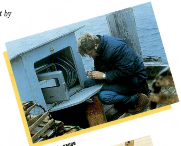
Checking tide gauge
