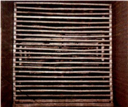
Trolley of fish in tunnel dryer
