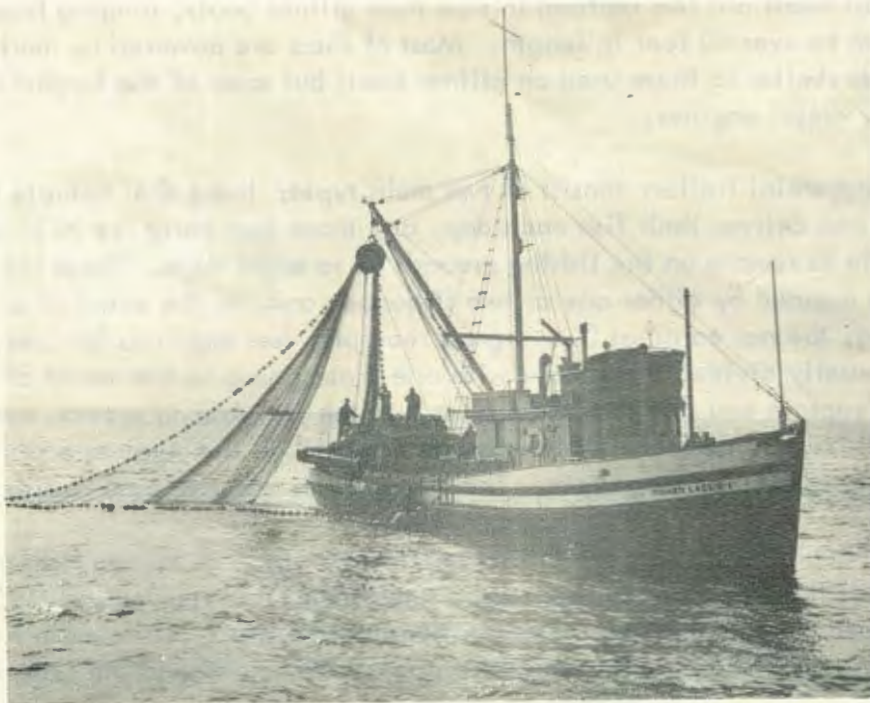
Figure 4. Purse-Seine Vessel (Table Type) Equipped with Hydraulic Block
