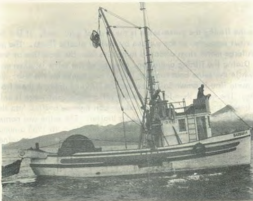
Figure 5. Purse-Seine Vessel (Drum Type)
