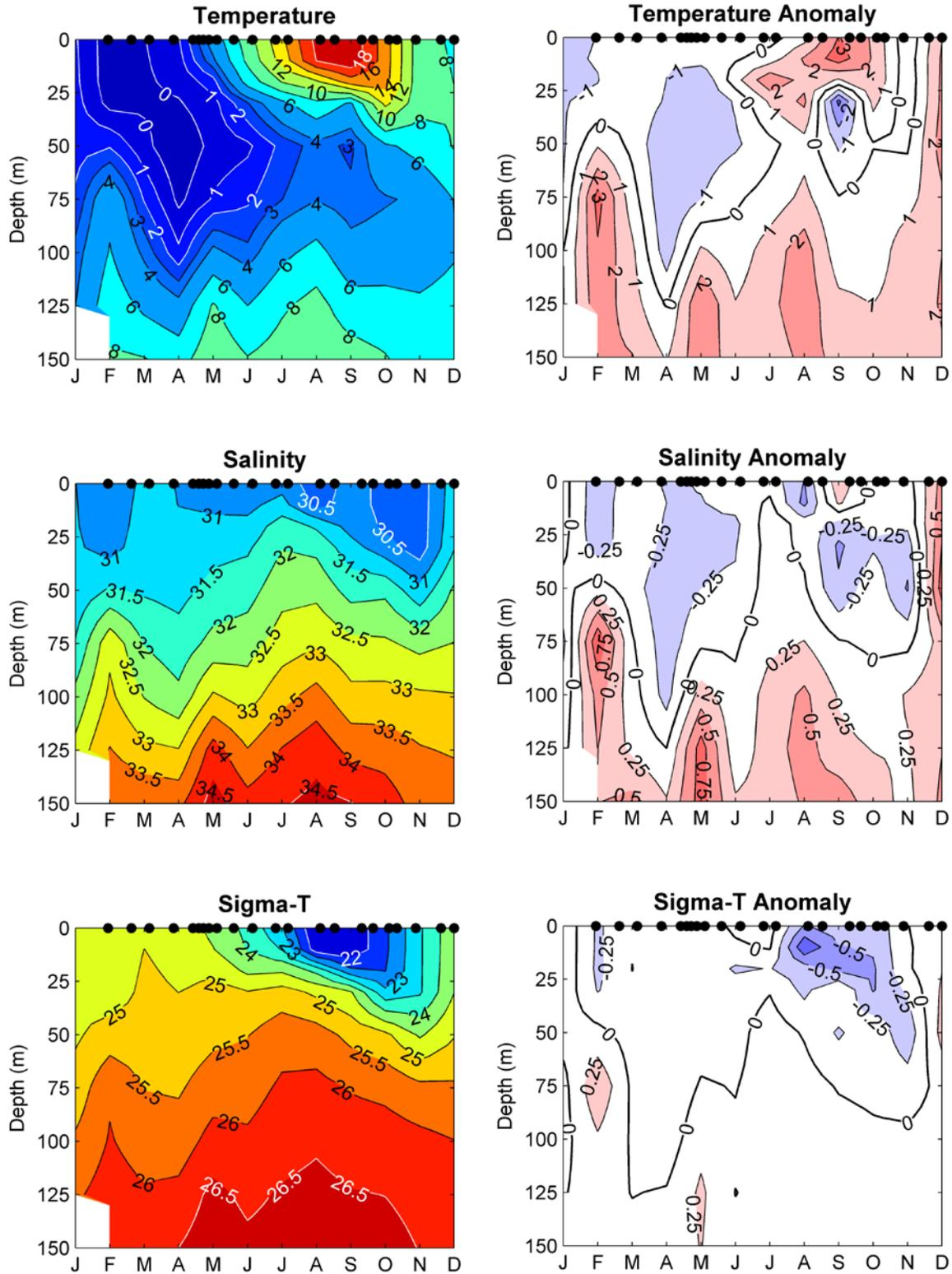
Figure 19. The 2015 annual cycle of temperature (top panel), salinity (middle panel) and density (lower panel) and their anomalies with respect to 1981-2010 monthly means (right panels) for Halifax station 2. Bullets indicate periods of sampling.
