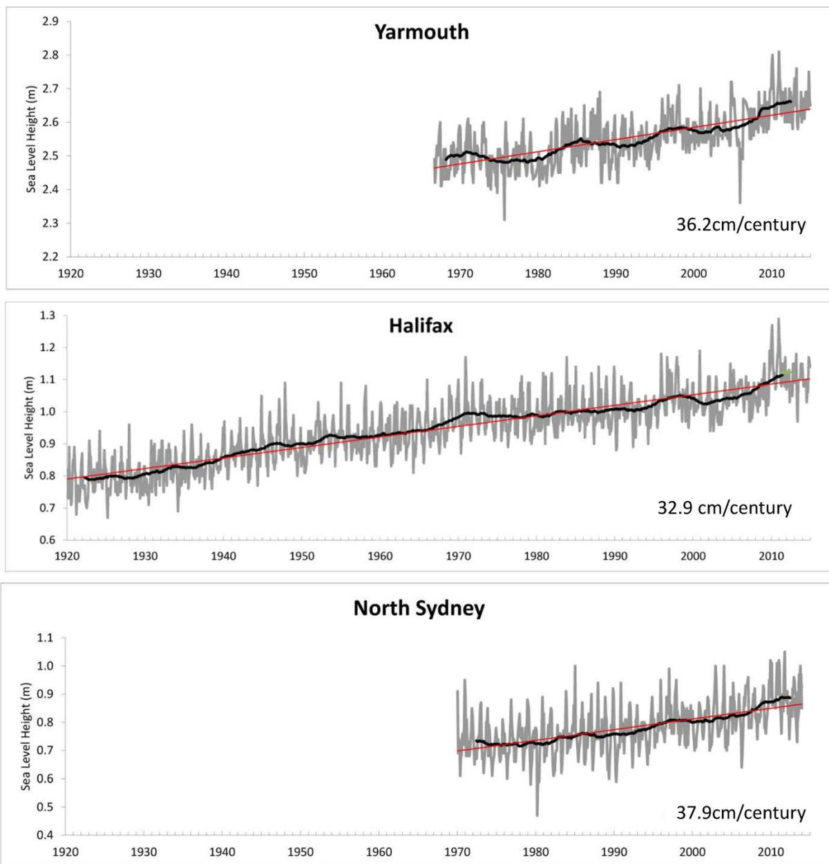
Figure 31. The time series of the monthly means (grey line) and a five year running mean (black line) of the relative sea level elevations at Yarmouth (top panel), Halifax (middle panel) and North Sydney (bottom panel), along with the linear trend (red line) over the observation period.
