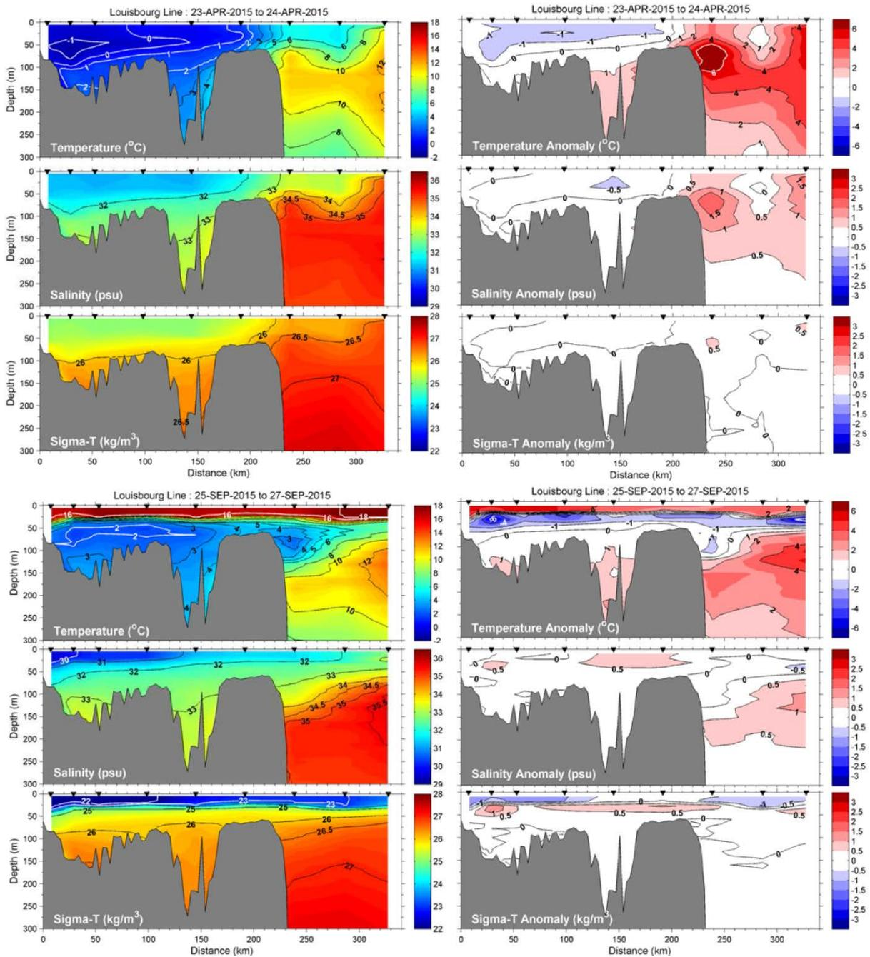
Figure 22. The 2015 sampling of the Louisbourg Line for Spring (top three panels) and Fall (bottom three panels). Temperature (top panel in each group), salinity (middle panel in each group) and density (lower panel in each group) and their anomalies with respect to 1981-2010 monthly means (right panels). Bullets indicate periods of sampling.
