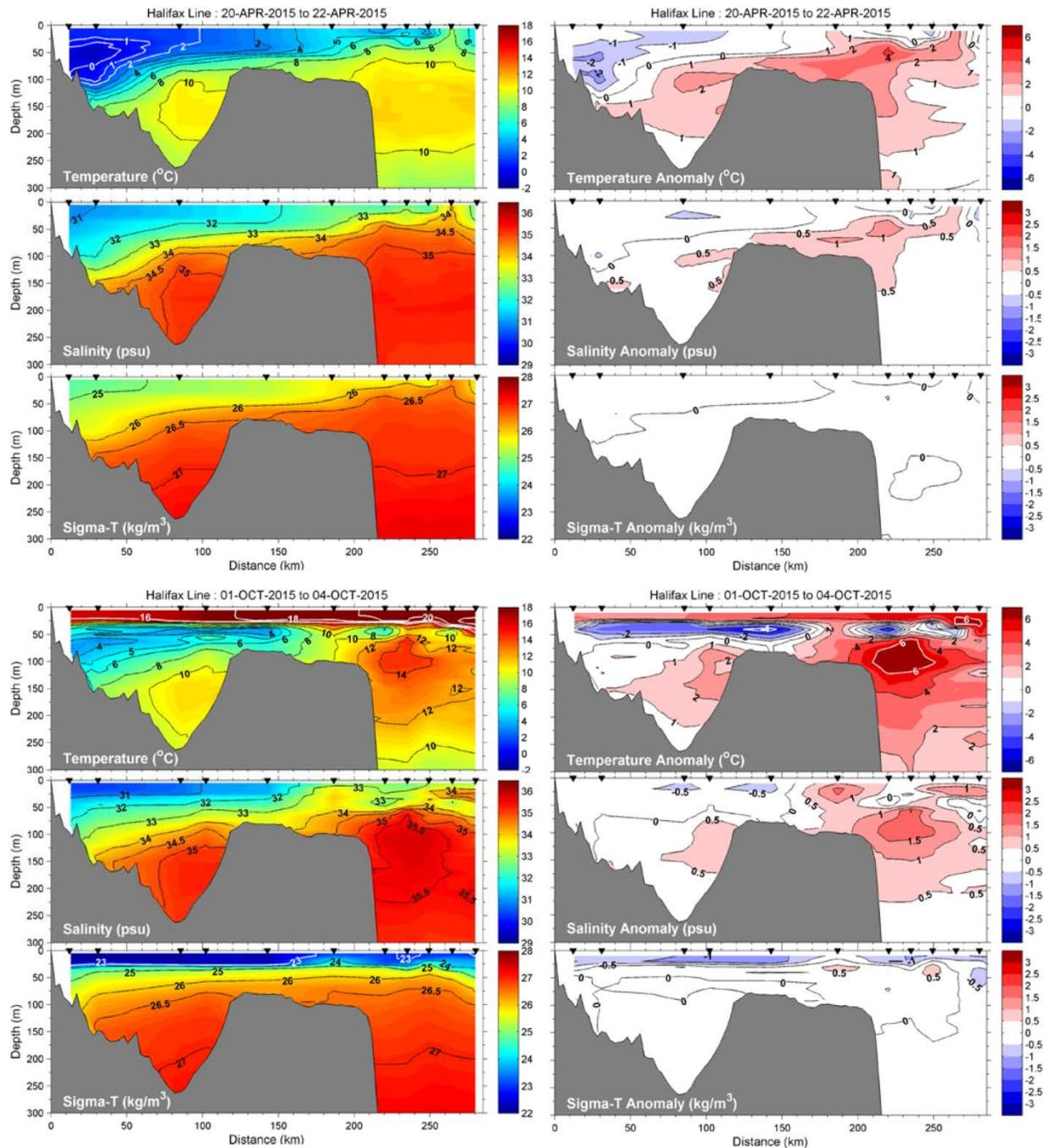
Figure 23. The 2015 sampling of the Halifax Line for Spring (top three panels) and Fall (bottom three panels). Temperature (top panel in each group), salinity (middle panel in each group) and density (lower panel in each group) and their anomalies with respect to 1981-2010 monthly means (right panels). Bullets indicate periods of sampling.
