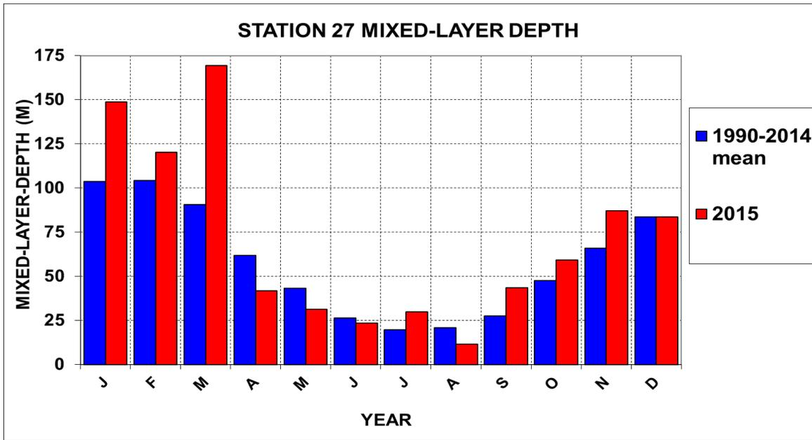
Figure 27. The 1990-2010 average and the 2015 monthly mean Mixed Layer Depths at Station 27.
