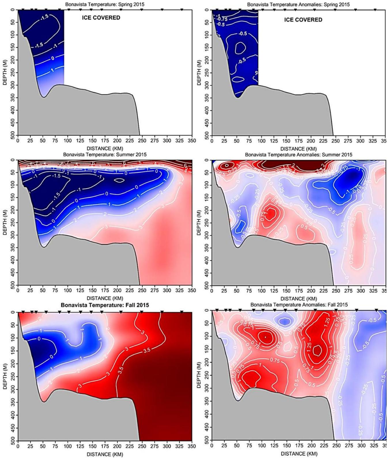
Figure 35. Contours of temperature ( $^{\circ}\text{C}$ ) and temperature anomalies along the Bonavista section (Figure 2) during the spring, summer and fall of 2015. Station locations along the section are indicated by the symbols on the top of each panel.
