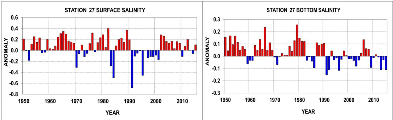
Figure 22. Annual Station 27 near-surface and near-bottom salinity anomalies referenced to the 1981-2010 mean. The mean and SD are shown in Figure 24.
