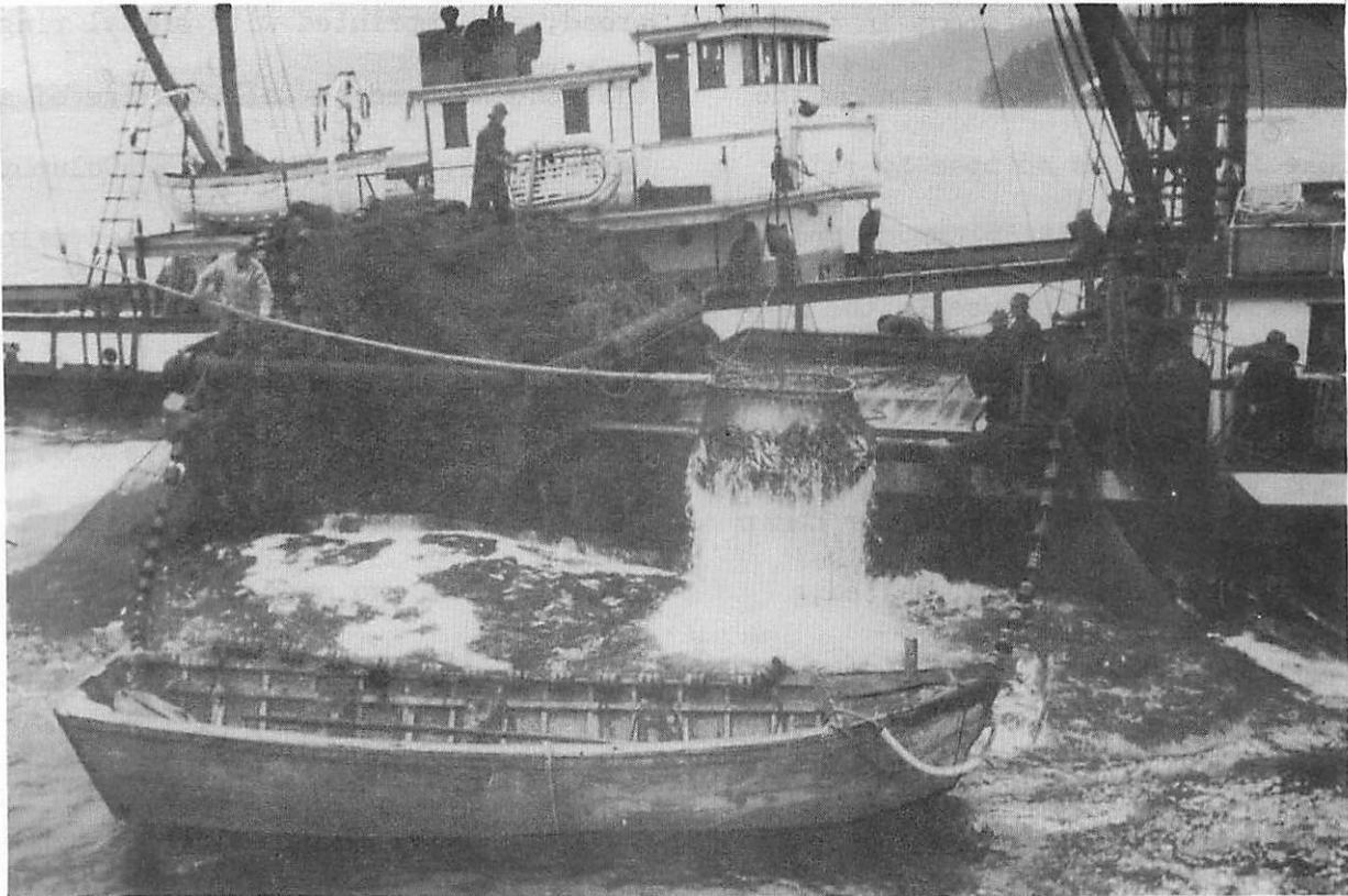
Fig. 3. HERRING HARVEST. The 70-80 foot fishing vessels may make catches of 100 tons or more. The silvery fish are transferred or brailled two tons at a time with a giant dip net into the hold of the fish boat.
