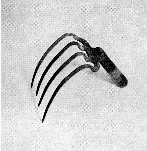
FIGURE 2. Bloodworm fork. The tynes are 9 to  $10\frac{1}{2}$  inches long, tapering from  $\frac{3}{4}$  inch at the base to  $\frac{1}{2}$  inch near the tip. Most diggers have them made from ordinary garden forks. (Photo by P. W. G. McMullon).
