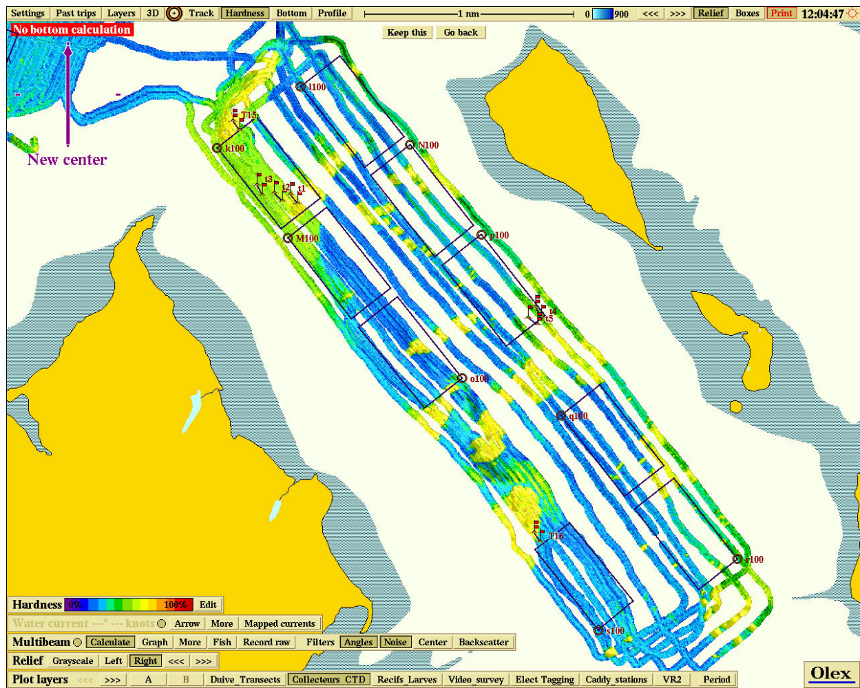
Figure 11. Hardness coefficients of the sites below Courtin Island (south block) from the acoustic seabed survey conducted in Malpeque Bay, PEI. The hardness classification is from hard (>90%; red) to soft (<25 %; dark blue). Map includes the proposed shellfish aquaculture sites (open polygons) and location of SCUBA transects (red flags: T1-5, 15 and 16).
