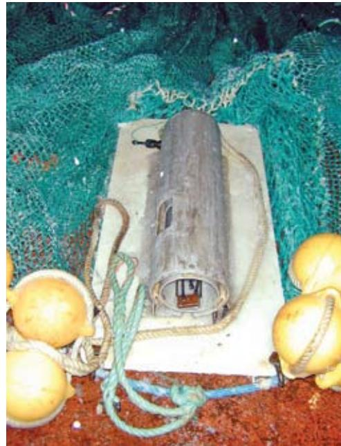
Fig. 2 The trawl-mounted CTD package ready for deployment.
