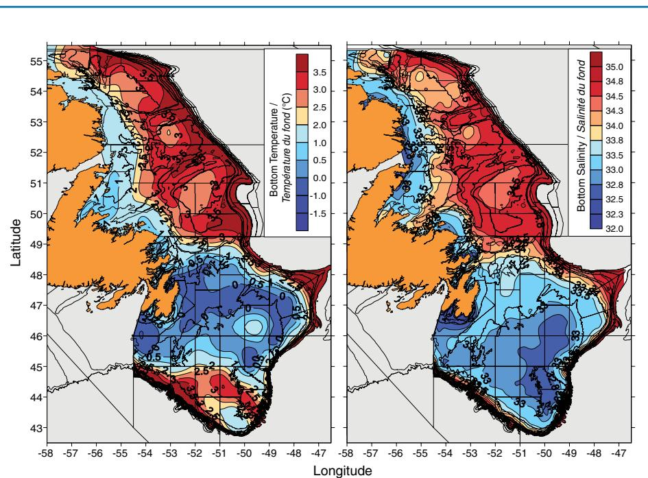
Fig. 4 Bottom temperature and salinity maps derived from the trawl-mounted CTD data from about 700 fishing tows in 2JsK3LNO during the fall 2005 multi-species survey.
