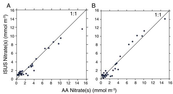
Fig. 5 Relationship between corrected ISUS optical estimates of nitrate concentration determined by UV spectrophotometry and conventional Technicon autoanalyzer (AA) measurements: (A) offset-corrected values and (B) temperature-corrected values made by increasing the ISUS nitrate values by the same proportion as the error in optical salinity. Both corrections of the optical estimates are highly correlated ( $r = 0.97$ ) with laboratory measurements.
