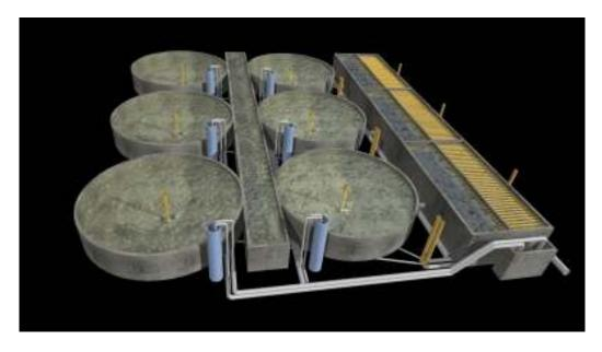
Figure 4. Schematic Drawing for One Fish Production Module
