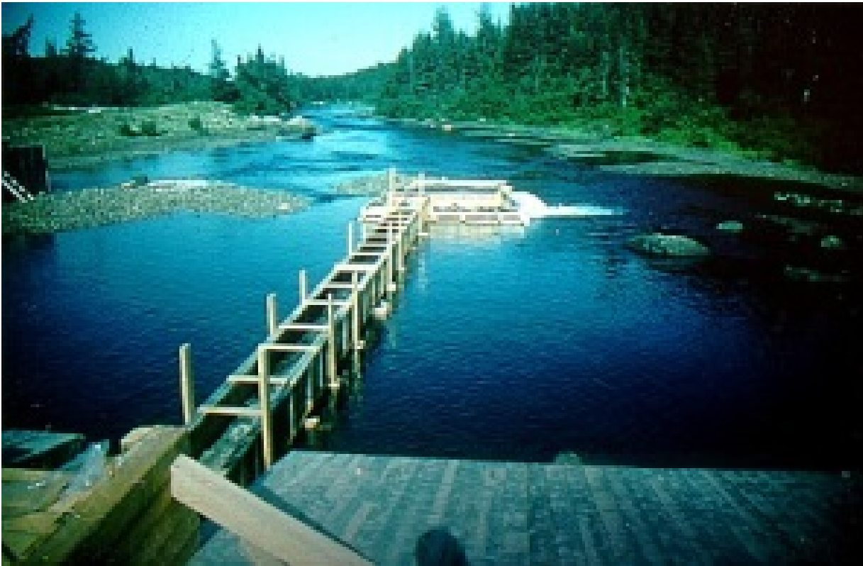
Figure 1. An example of a volitional flume. This temporary experimental open channel was constructed at the Noel Paul's Brook Research Facility in central Newfoundland, Canada (photo by M. Colavecchia). Published swim data obtained from this and various others types of experimental set-ups were included in the database compiled and used in this study to develop fish swim performance curves.
