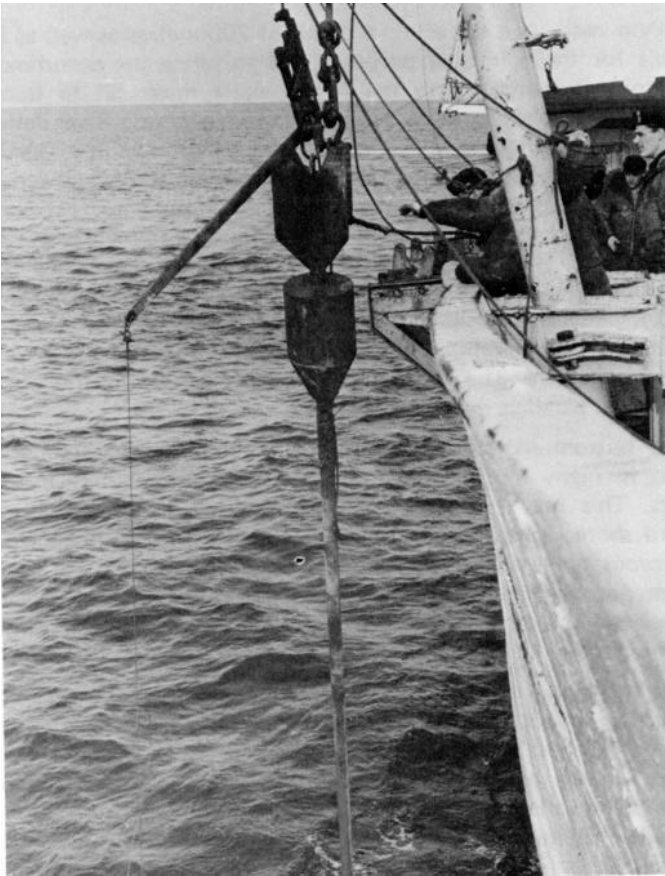
Piston corer being used from the CSS Hudson in Beaufort Sea.
