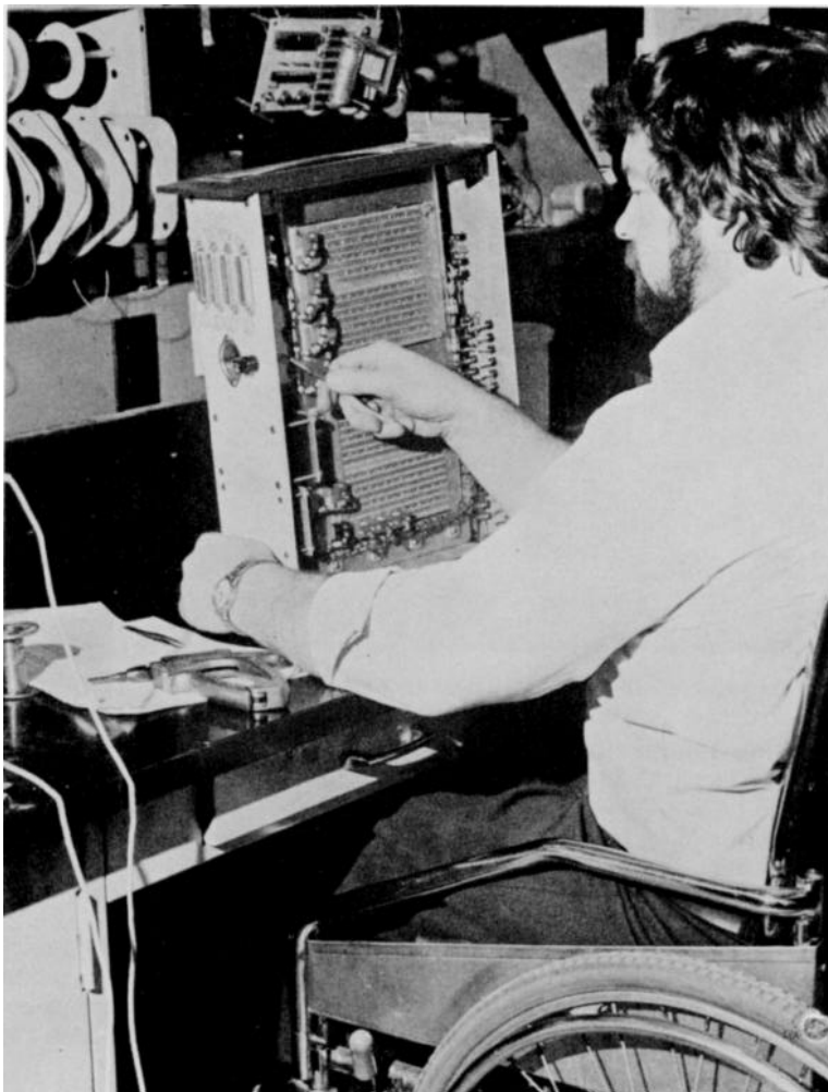
Technician wiring and assembling an electronic chassis. (AOL 3446.)
