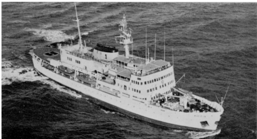
The CSS Baffin is a diesel-driven ship designed primarily for hydrographic survey work in arctic waters. She is used for offshore hydrographic charting and geophysical studies and for survey work in coastal and arctic waters. The vessel is ice-strengthened, has a cruising range of 22,400 kilometres and 45 days endurance, and carries five hydrographic survey launches and geophysical recording instruments. (AOL 3093-2.)
