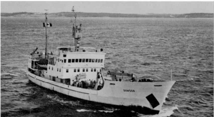
The CSS Dawson is a diesel-driven ship designed and used for oceanographic work in offshore as well as coastal waters. She has a cruising range of 19,200 kilometres and 60 days endurance. The vessel is equipped with a bowthruster and controllable pitch propellers and is particularly well suited for placing and retrieving moored buoys and instruments. (AOL 1727-51.)
