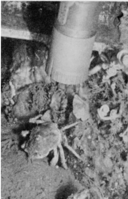
The underwater electric rock core drill is used for continental shelf exploration and can be operated from an oceanographic research vessel.
