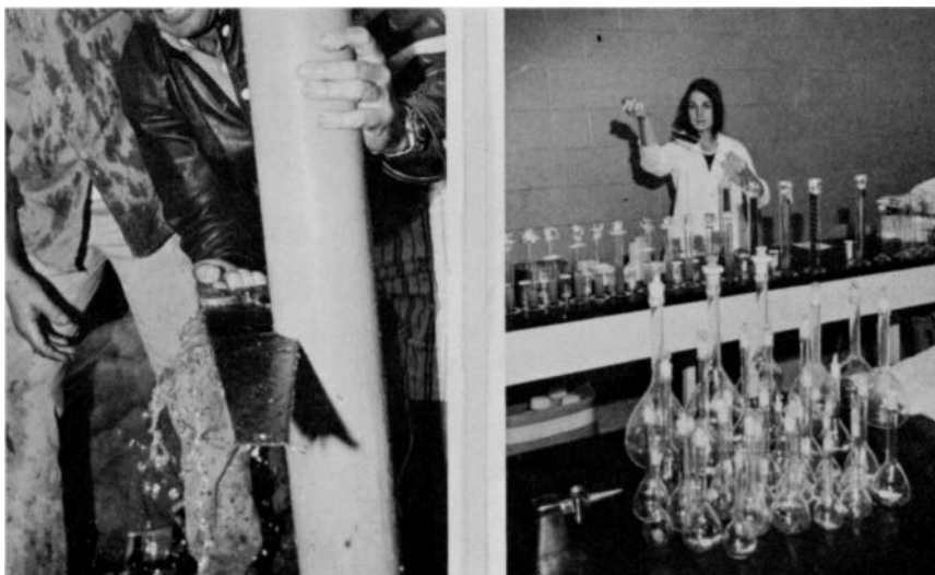
Sawing through the protective core barrel prior to removal of the Canso Strait sediment core within. Later these cores were subjected to various chemical analyses. (AOL 2835-235 and - 169 )
