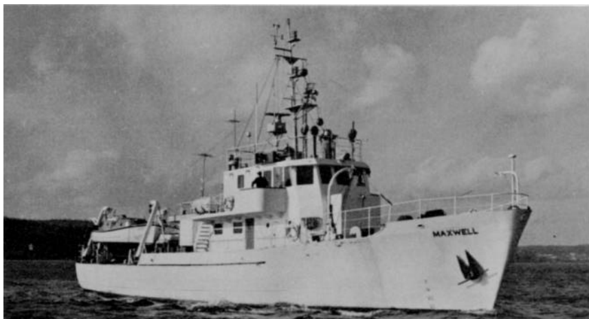
The CSS Maxwell is a diesel-driven ship designed for hydrographic work in nearshore and coastal waters. She has a cruising range of 3200 kilometres and 14 days endurance, and carries two survey launches. The Maxwell is utilized mainly for hydrographic charting along the coasts of the Atlantic provinces. (AOL 2637-4.)
