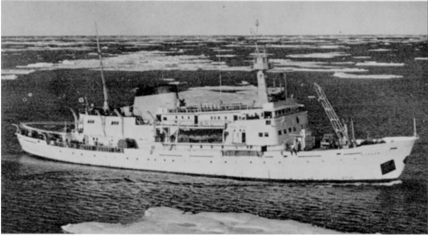
The CSS Hudson is a diesel-electric driven ship designed as a combined oceanographic research and hydrographic survey vessel. She is primarily utilized for multi-disciplinary offshore oceanographic surveys ranging from tropical to arctic waters. The vessel is ice-strengthened, has a cruising range of 24,000 kilometres with 60 days endurance, and is equipped with a bowthruster, scientific laboratory facilities, and recording instruments. (AOL 1727-51.)
