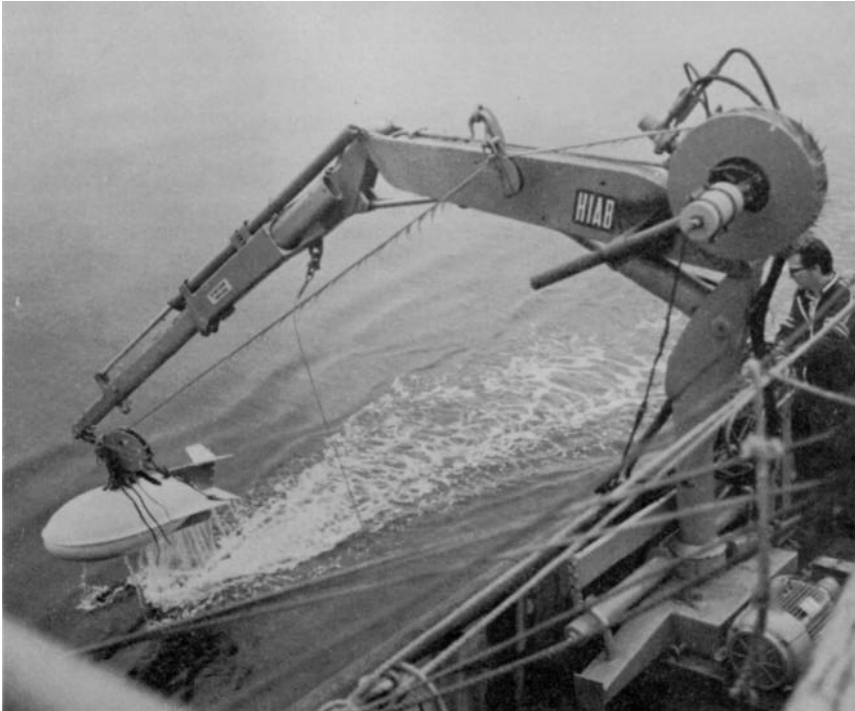
A hydraulic crane is used to lower and raise the CECS towed body, which contains the echo sounder's transducer. (AOL 2535-5.)
