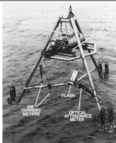
RALPH is the name of an instrument package developed and built by the Atlantic Geoscience Centre to study coastal sediment features and the mechanics of sediment transport.
