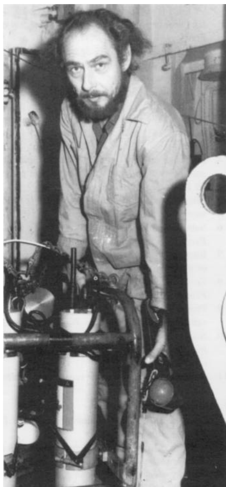
Heinz Wiele prepares the deep-sea camera assembly for lowering over the side of C.S.S. Hudson.
