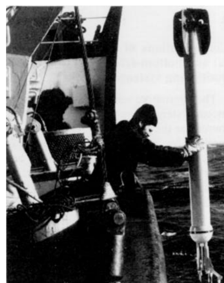
The OCTUPROBE being deployed from the C.S.S. Dawson during a recent study of the spatial variability of turbulence in the mixed layer.
