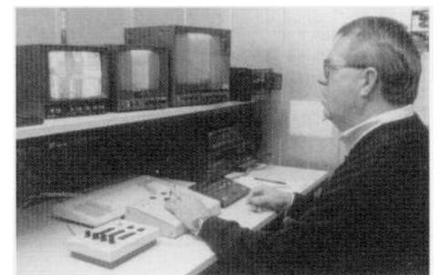
Figure 3: Photograph of the AGC X-Ray system. Cores are placed vertically into a computer controlled track which remote\ moves and rotates the whole core while the operator views the X-ray data on a video display monitor.
