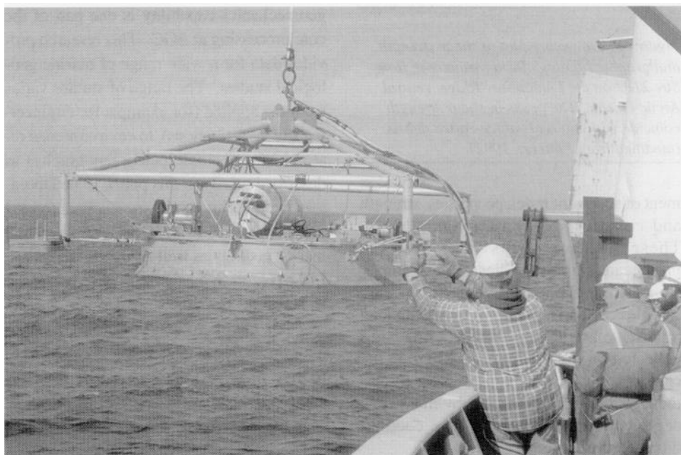
Figure 2: Sea Carousel, an AGC developed in situ flume being deployed from CSS Hudson in Hudson Bay. The annular flume, equipped with optical backscatter sensor and a video recorder is used to simulate near-bed flows and initiation of sediment transport.
