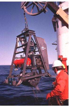
*Figure: 4. Videograb (with DRUMS attached) which collects organisms living on and in the seabed (samples 0.5 m<sup>2</sup>).*
