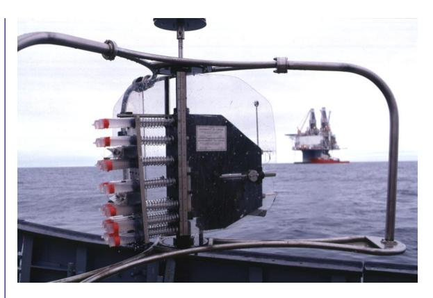
*Figure 3: BOSS being recovered after sampling near the Hibernia Platform on the Grand Banks. Suspended sediment samples are collected from the benthic boundary layer by spring loaded syringes at 7 depths between 5 and 50 cm above the sea floor.*
