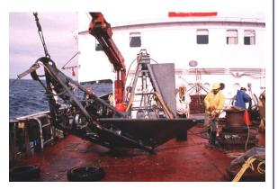
Figure: 3. Epibenthic sled which collects large organisms living on the seabed (samples approximately  $18 \text{ m}^2$  on a 50 m tow).
