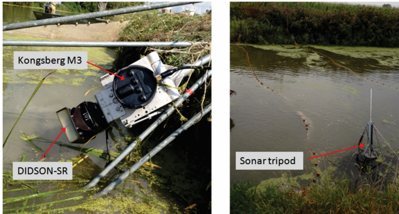
Figure 4. DIDSON sonar and Kongsberg sonar units mounted on adjustable tripod frame (left image). Sonar tripod deployed within isolation net enclosure (right image). Source: Milne Technologies.
