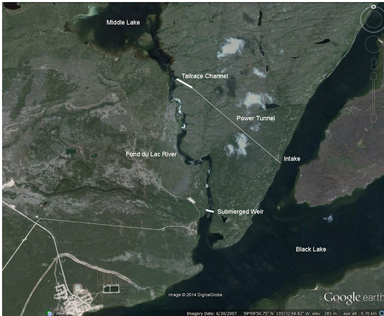
Figure 1. Map of the Fond du Lac River between Middle Lake and Black Lake (from Google earth). Approximate locations of the proposed Taxi Twé Hydroelectric Project's submerged weir, water intake, power tunnel and tailrace channel are identified.
