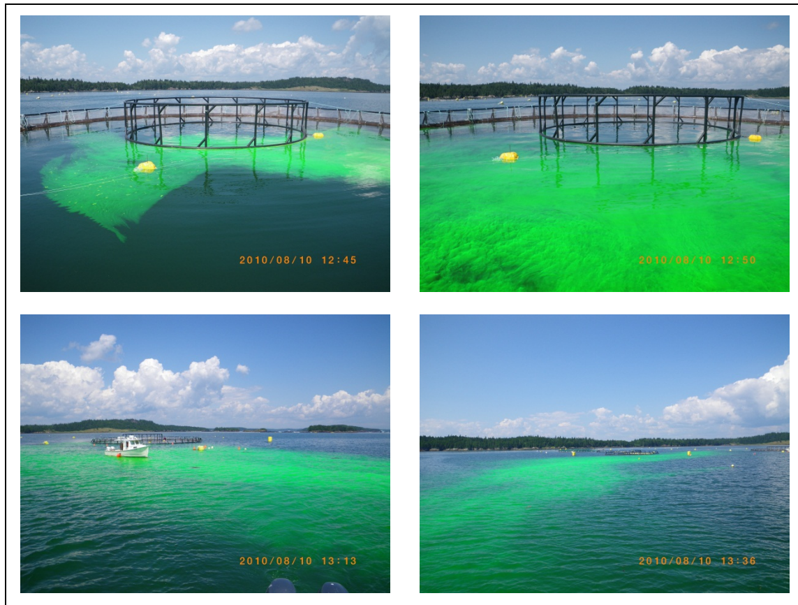
Figure 15. Pictures showing the evolution of the dye plume resulting from a dye release from Site A on the 10 th of August 2010.
