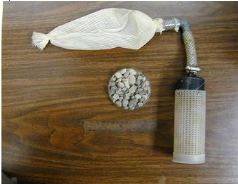
Figure 8. Details of a) egg capsule injection device disassembled with a capsule, b) assembled egg capsule injection device, and c) egg capsule with emergence collection net attached and sample of substrate used.
