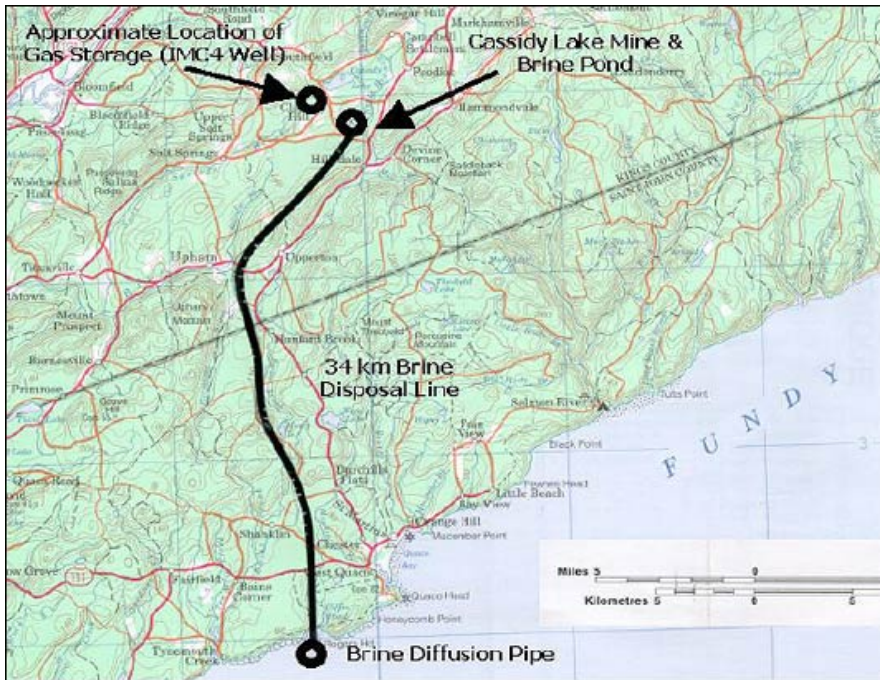
Figure 10: Sketch of southern NB and approximate location of potash brine disposal pipeline from Cassidy Lake, NB, to the Bay of Fundy
