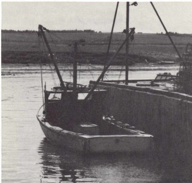
Typical lobster boat, rigged with twin booms for Chondrus harvesting off Skinner's Pond, Prince Edward Island, showing drag rakes on the roof and along the gunwale.
