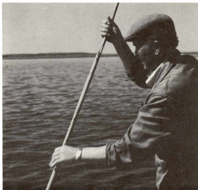
Using a pole to determine bottom firmness, during assessment of area's suitability for oyster growing.
