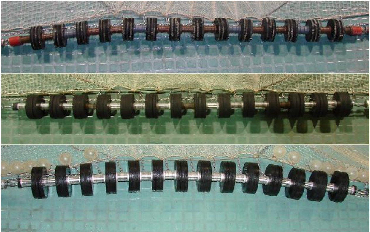
Figure 1. Center bosom section of the three model footgears tested representing 14" (top), 18" (middle) and 21" (bottom) rockhopper disks.
