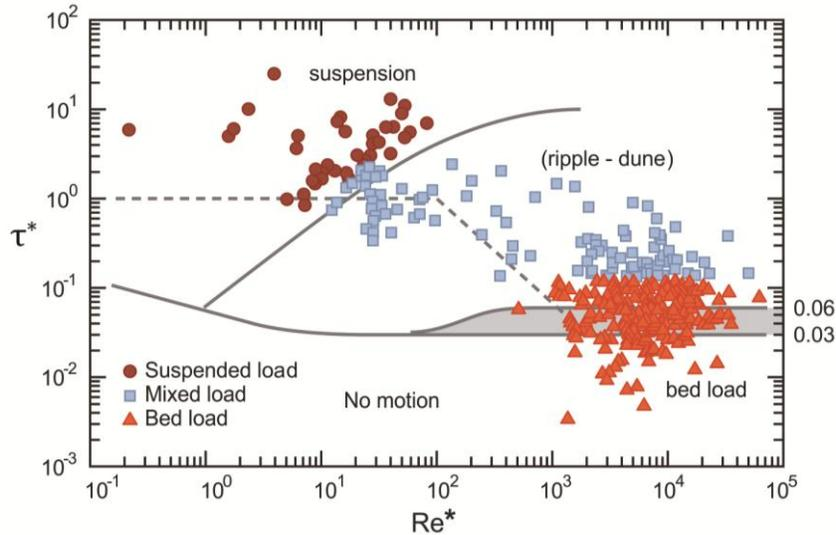
Figure 10. Shields stress and Reynolds number ( $Re^* = \mu^* D / \nu$ , where  $\mu^*$  is the shear velocity,  $\nu$  is the kinematic viscosity of water, and  $D$  is grain size) in suspended load, mixed load, and bedload streams (from Church 2006).
