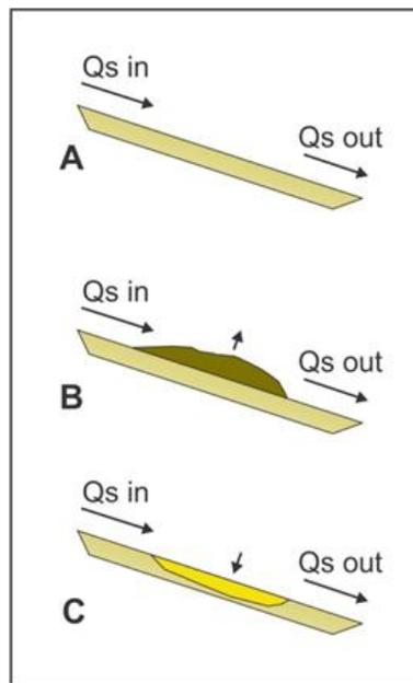
Figure 3. (A) Downstream sediment discharge patterns for a stable river bed that is in grade ( $Q_{s\ in} = Q_{s\ out}$ ). (B) Downstream sediment discharge patterns for an aggrading river bed ( $Q_{s\ in} > Q_{s\ out}$ ). (C) Downstream sediment discharge patterns for a degrading river bed ( $Q_{s\ in} < Q_{s\ out}$ ). (from Burge and Guthrie 2013).
