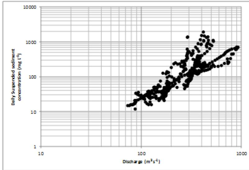
Figure 8. Relationship between suspended sediment concentration and discharge for the Mackenzie River East Channel at Inuvik (Data from the years 1975 – 1977 and 1994 for WSC 10LC002;  $k = 0.0075$  and  $b = 1.7441$ ).
