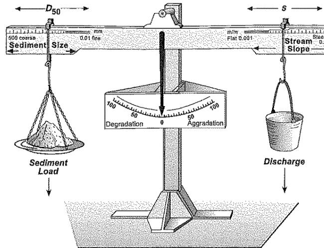
Figure 2. Diagram of Lane's Law showing the driving forces on the right side of the scale and the resisting framework on the left side of the scale (from Fryirs and Brierley 2013).
