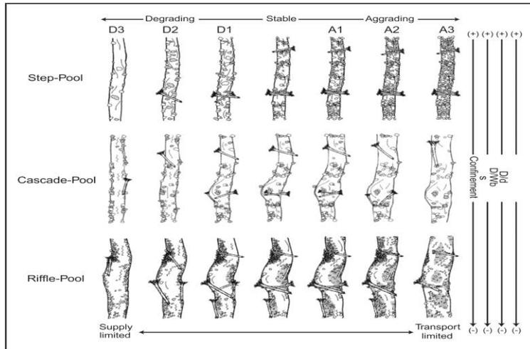
Figure 13. Channel morphology matrix showing effects of increasing sediment input on step-pool, cascade pool, and riffle pool channels (British Columbia Ministry of Forest and British Columbia Ministry of Environment 1996).
