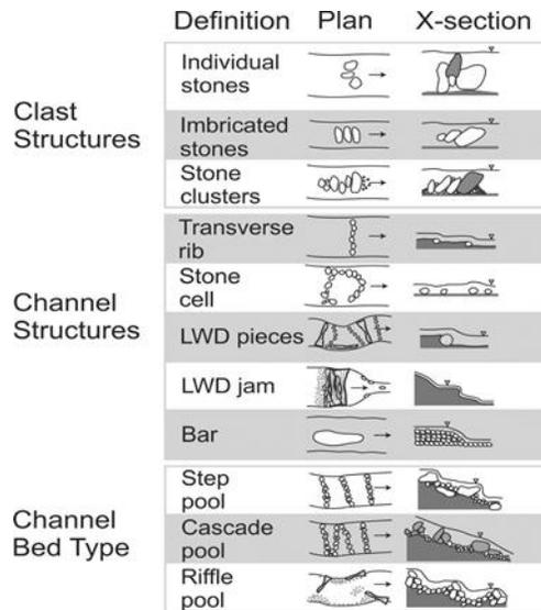
Figure 12. Channel elements at the micro- to meso-scale (Hassan et al. 2008).
