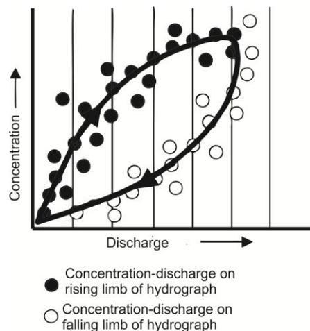
Figure 7. Generalized hysteresis curve for suspended sediment concentrations showing the rising limb of the hydrograph with higher concentrations than the falling limb.
