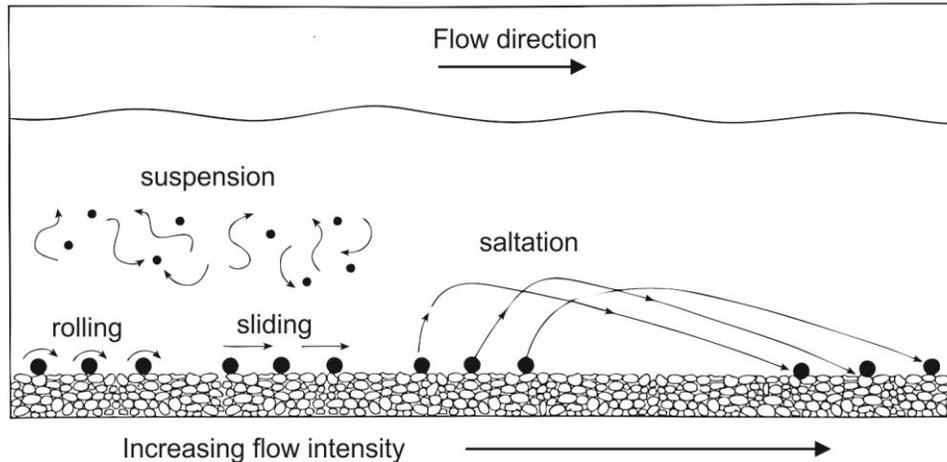
Figure 1. Cartoon diagram showing rolling, sliding, saltation and suspension of fluvial sediment [after Fryirs and Brierley (2013)].
