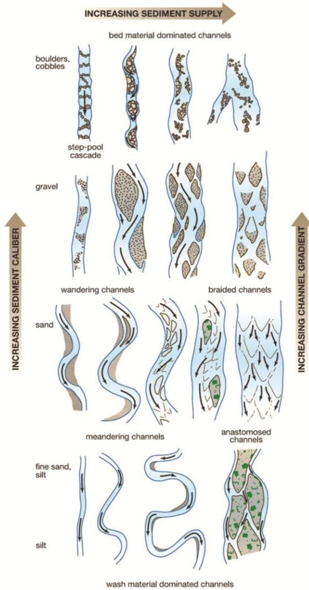
Figure 11. Channel patterns in relation to grain size, gradient, and sediment input (from Church 2006, modified from Mollard 1973, Schumm 1985, and Church 1992).
