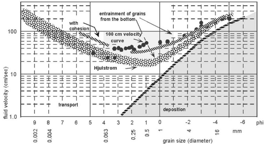
Figure 6. Curve by Hjulstrom (1939) showing the zones of entrainment, transport and deposition for a given velocity and grain size.
