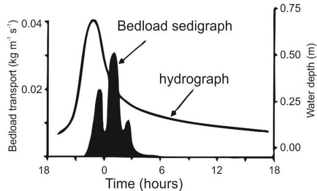
Figure 4. Example of bedload pulses measured on Turkey Brook in southern England (from Reid et al. 1985 and Thorne et al. 1997).
