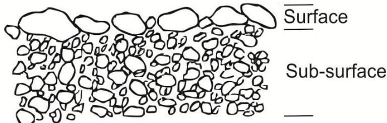
Figure 5. Cartoon drawing showing the surface and subsurface layers in a gravel-bed river (from Fryirs and Brierley 2013).
