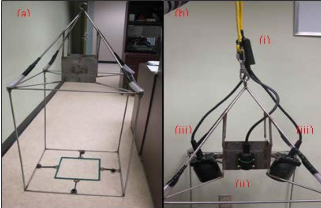
Figure 2. Bare camera frame with quadrants.
