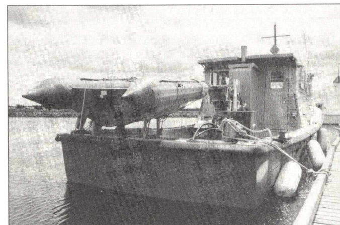
The J. WILLIE DERASPE is equipped with a 13-foot Avon boat and a winch which can haul up any kind of fishing gear used in the Magdalen Islands.
