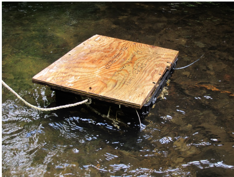
Figure 3. Milk crate trap with straw and lid used in lamprey studies
