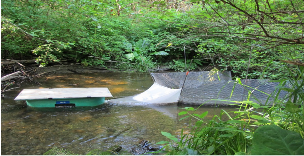
Figure 1. Photograph of live capture downstream lamprey trap installed in Morrison Creek, 2012 (J. Wade)
