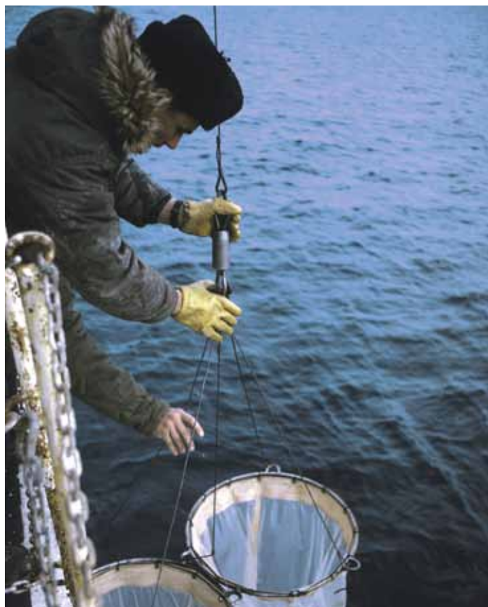
Lowering plankton nets to sample drifting organisms in the marine water column
