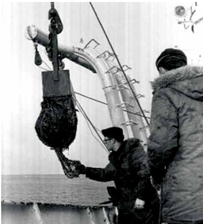
A dredge haul from the seabed surface is brought on board for analysis.
