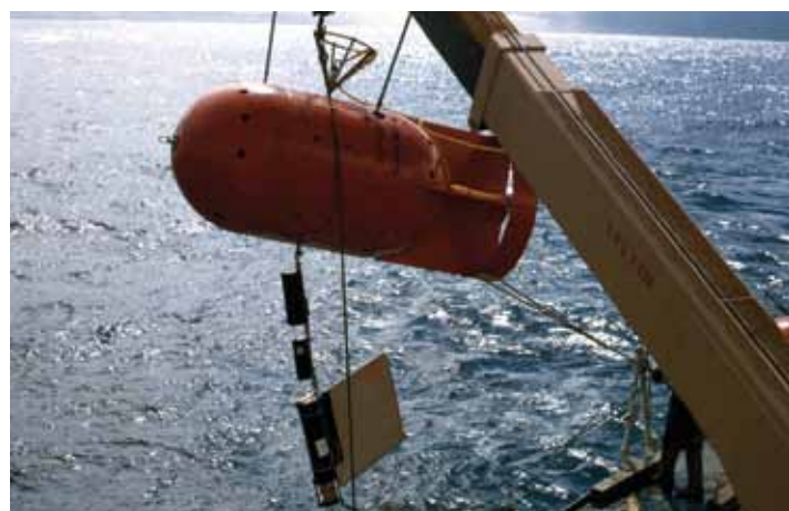
Deployment of current meter array in Drake Passage
