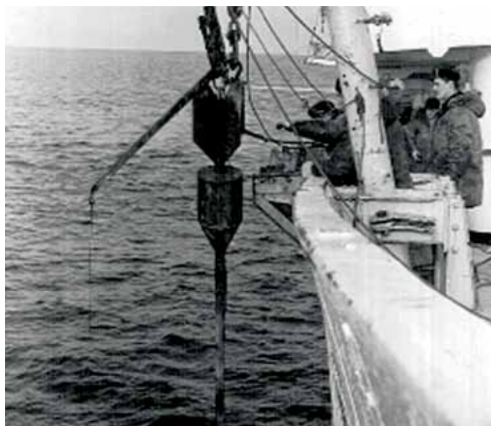
Crew deploys a corer to investigate sedimentation history in the Beaufort Sea.
