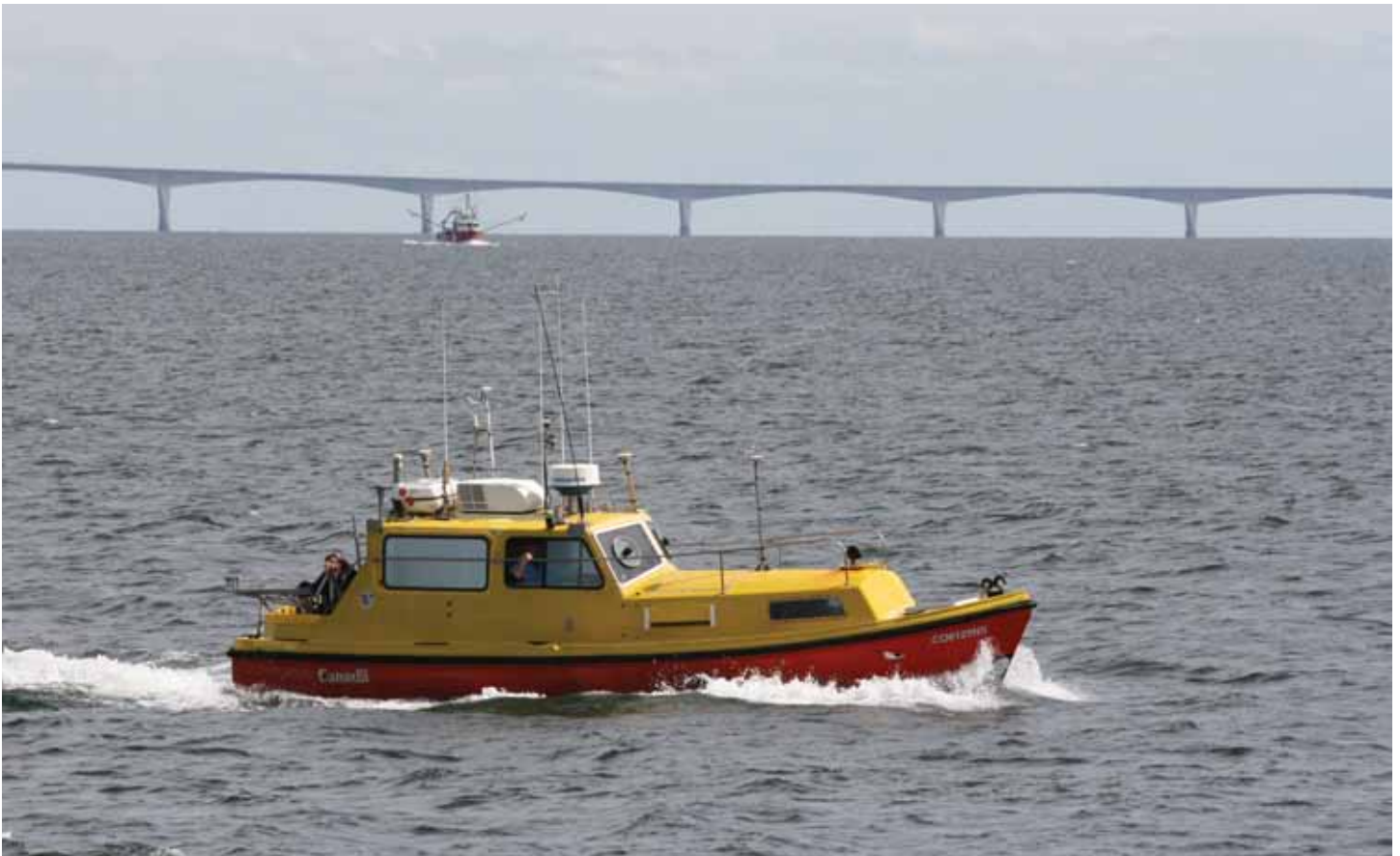
In 2009 the CCGS Matthew and her two launches conducted a hydrographic survey operating out of Summerside, Prince Edward Island. The multibeam seabed survey was in support of DFO Gulf Region's Ecosystem Research Initiative. This initiative included mapping Northumberland Strait on both sides of the Confederation Bridge. Pictured here is the Matthew's multibeam-equipped survey launch Plover in the foreground and in the background the CCGS Opilio conducting a benthic sampling survey. Photo courtesy of Mike Lamplugh
