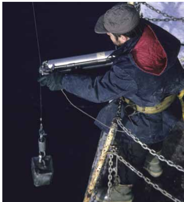
Recovering a bottle of sea water from a known depth for chemical analysis
