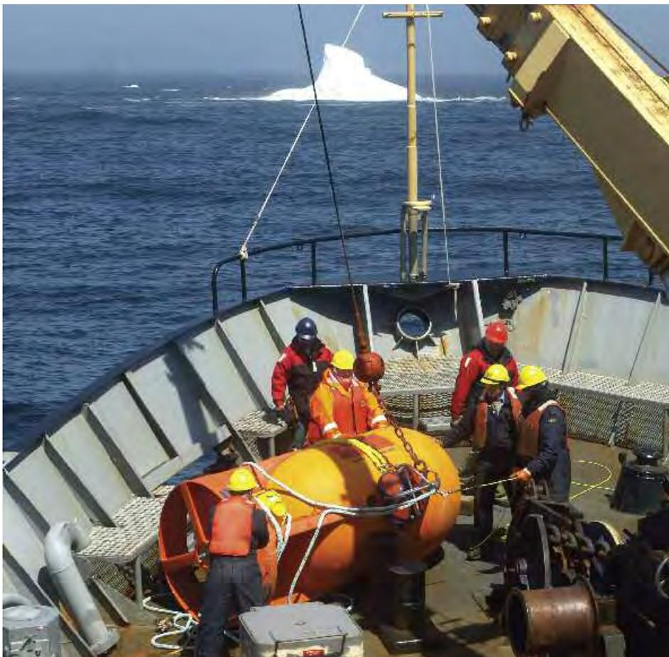
Figure 3a. A top float from a subsurface oceanographic mooring being secured on the deck of CCGS Hudson during a mooring recovery operation, Orphan Basin, May 2009 (image courtesy of Anthony Joyce)
