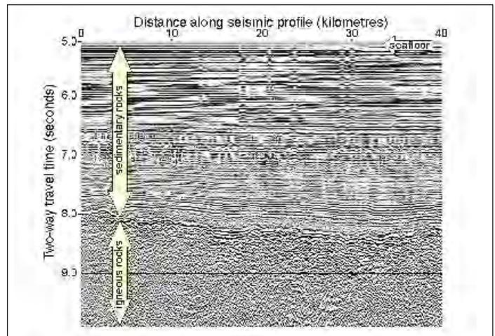
Figure 3. Example profile of the high quality seismic reflection data collected during the 2008 joint program with the CCGS *Louis S. St-Laurent* and the USCGC *Healy*
