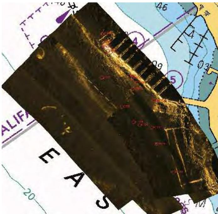
Example of a Halifax Force Protection survey of Naval Jetty NS located at Fleet Diving Unit Atlantic: the red circles indicate objects meriting further investigations.
