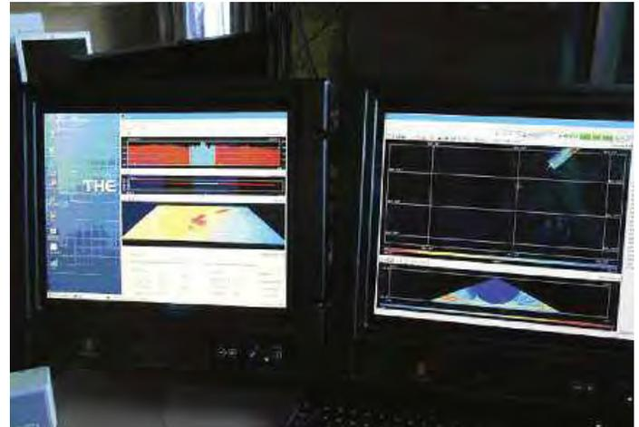
Operator console aboard the CCGS *Matthew* during multibeam acquisition
