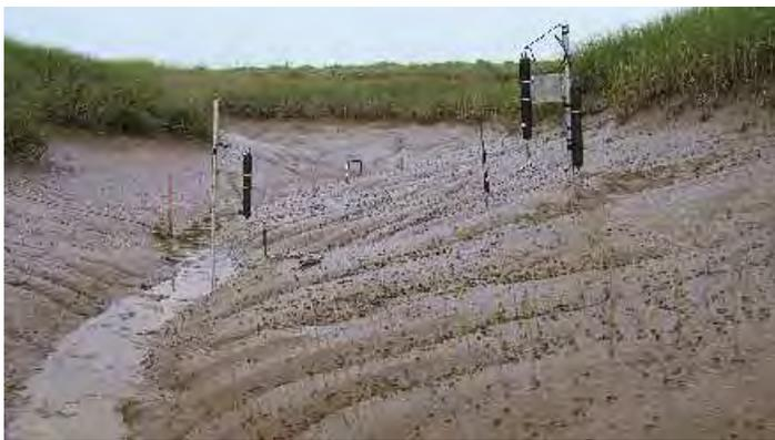
Figure 11. Sediment sampling array deployed in tidal channel of the Avon River, Windsor, Nova Scotia – photo courtesy of Dr. Danika van Proosdij, Department of Geography, Saint Mary's University
