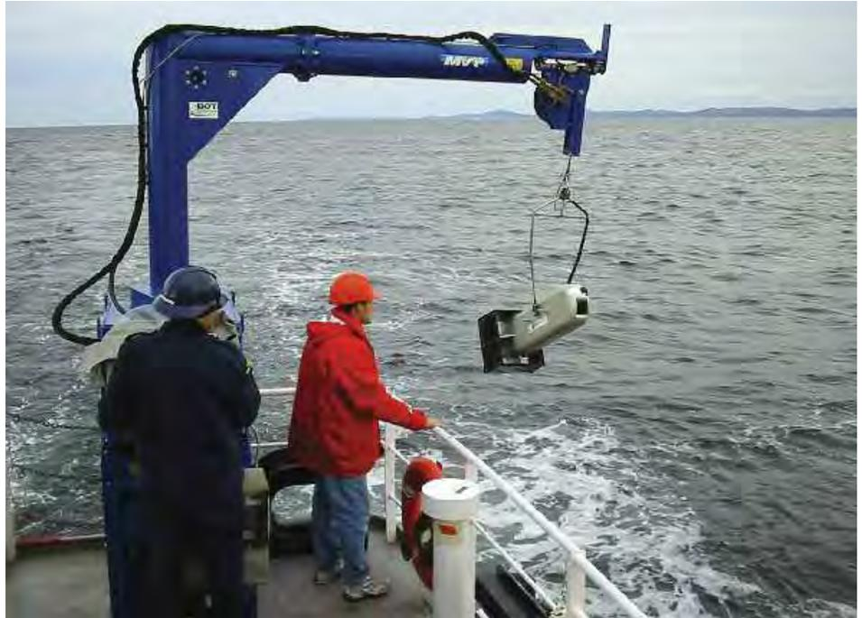
ODIM-Brooke Ocean MVP-200 Moving Vessel Profiler aboard the CCGS *Matthew*
