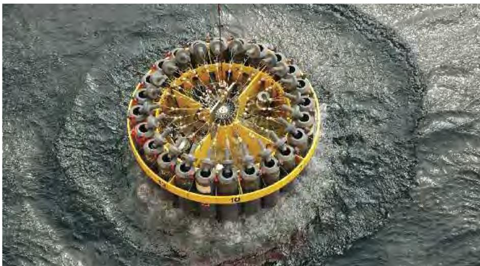
Figure 3b. Rosette system with water sampling "bottles" (around perimeter) and CTD system measuring key seawater properties (below surface and not visible) being lowered into water to do an oceanographic station in Orphan Basin of the Labrador Sea, May 2009 (image courtesy Igor Shkvoretz)
