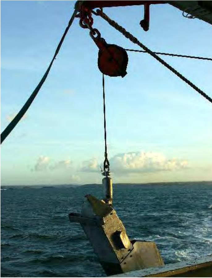
Figure 2a. Deploying a CPR – photo courtesy of SAHFOS
