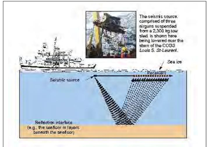
Figure 2. Schematic diagram of the system used to reliably collect seismic reflection data using icebreakers under a range of light-to-heavy ice conditions
