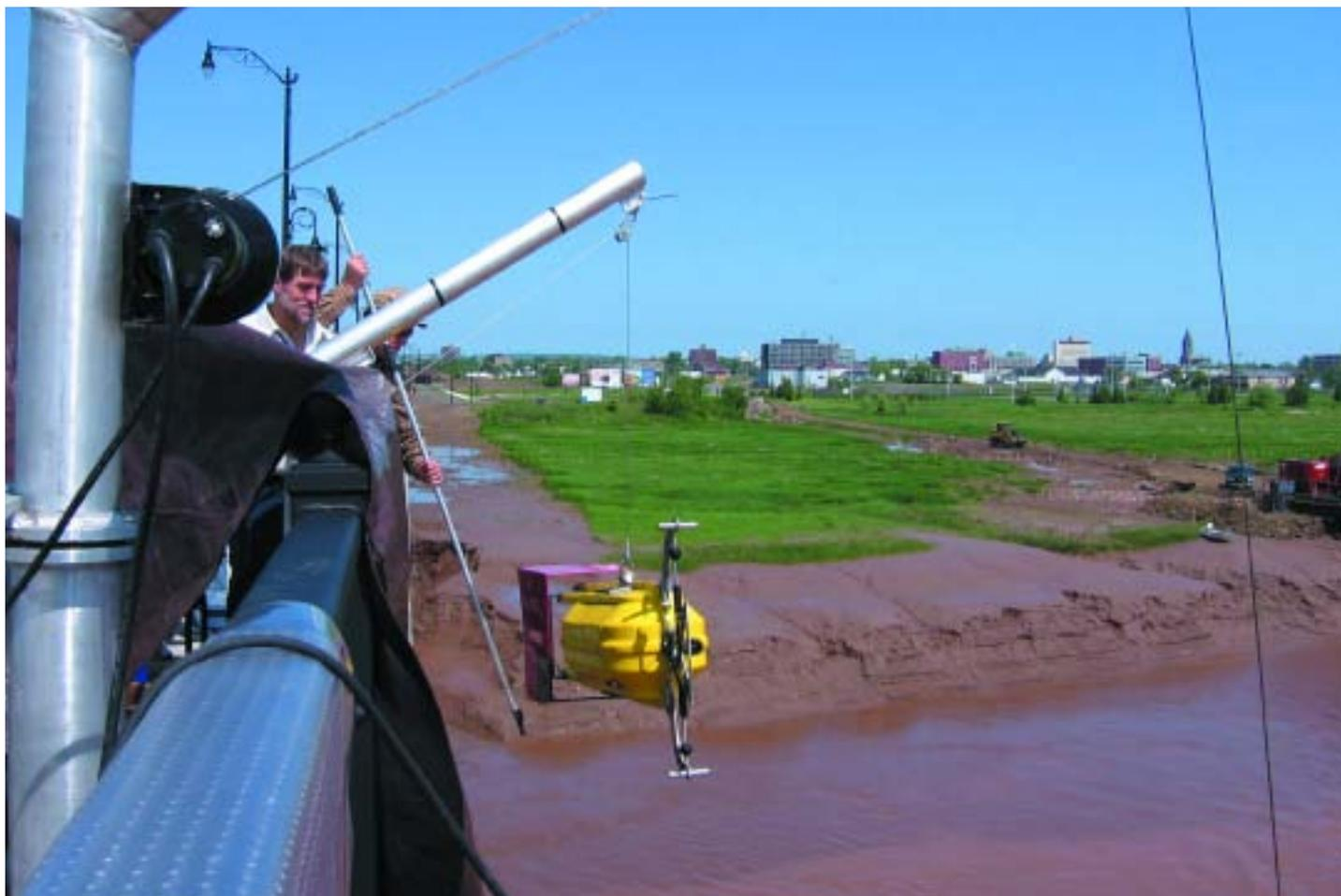
Tim Milligan and Paul Hill (behind davit) are deploying an instrument package from the Gunningsville bridge in Moncton, New Brunswick. The streamlined package contains a number of instruments designed to collect data on fluid mud in the Petitecodiac River.
