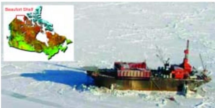
**Figure 1** SDC hybrid drilling platform on location in the Beaufort Sea at the Devon Paktoa C60 well site (photo courtesy of Devon Canada)
