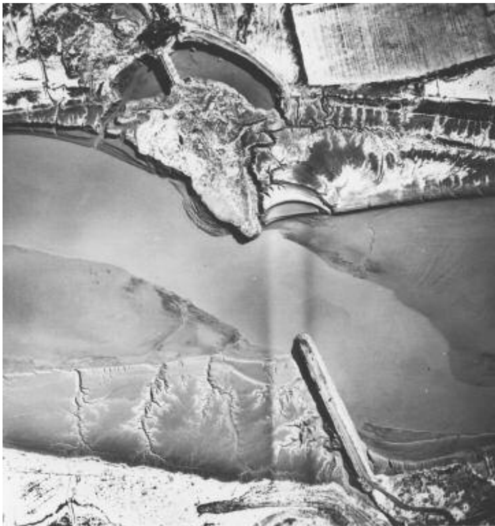
Figure 1. The Petitcodiac River causeway under construction: downstream is to the left. The mudflat is growing at the same pace as the causeway is extended.
