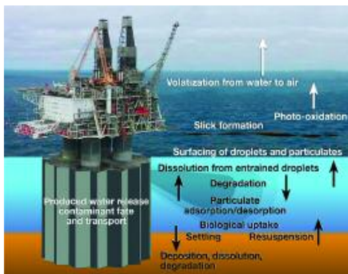
Schematic representation of the fate and contributing processes for production waters from Hibernia oil production platform
