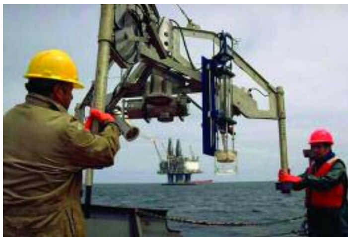
Deployment of a moored bottom tripod to measure sediment concentrations and other variables in the benthic boundary layer near the Hibernia structure
