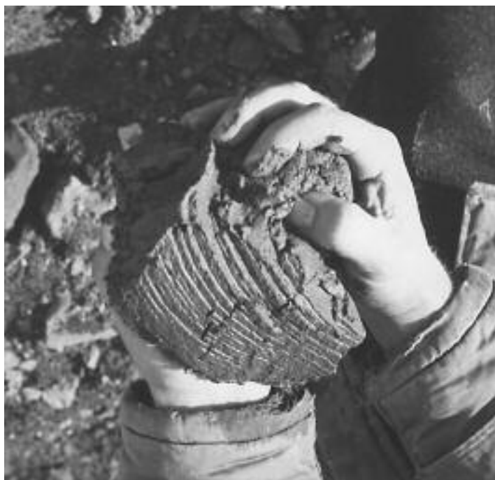
Figure 3. Sediment sample collected during causeway construction showing the layers deposited during each tide
