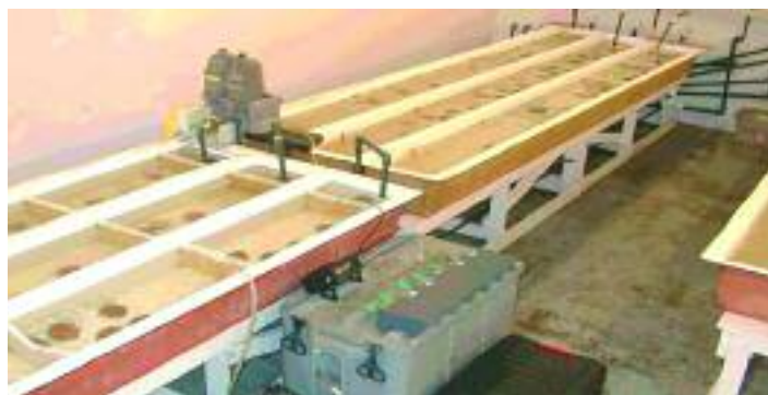
Flow-through tanks used in laboratory experiments of drilling-mud effects on sea scallops
