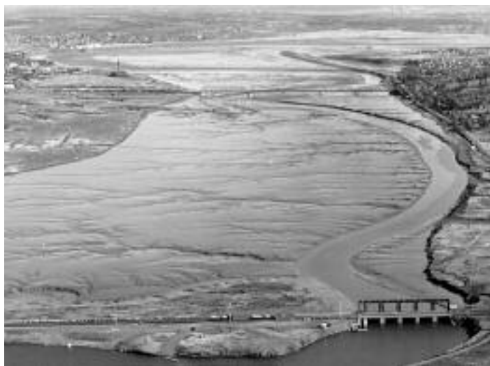
Figure 4. View downstream from the causeway showing the extensive new mud flats a year after causeway completion
