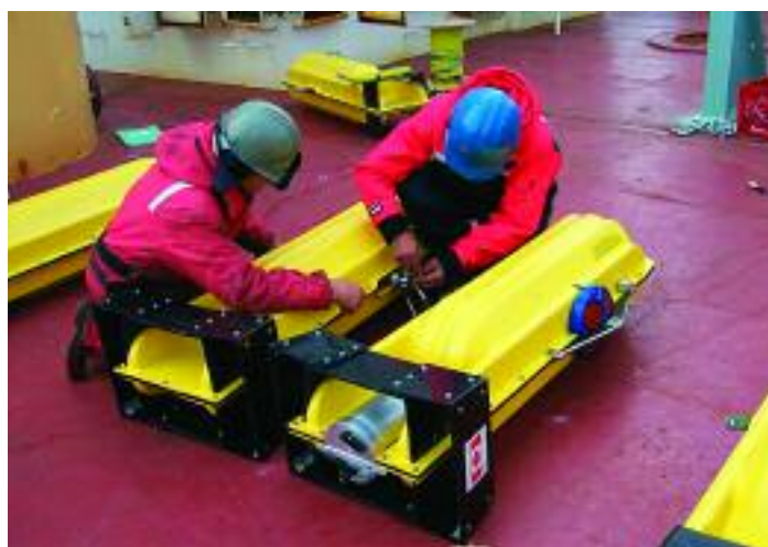
Figure 2. Mooring deployment preparations showing one of the instrumented buoyancy assemblies: the acoustic Doppler current profiler protrudes through the top of the package, while the compass is the silver cylinder mounted in the tail.
