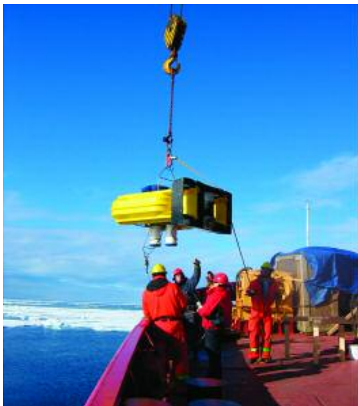
Figure 4. Deployment of an instrumented mooring
