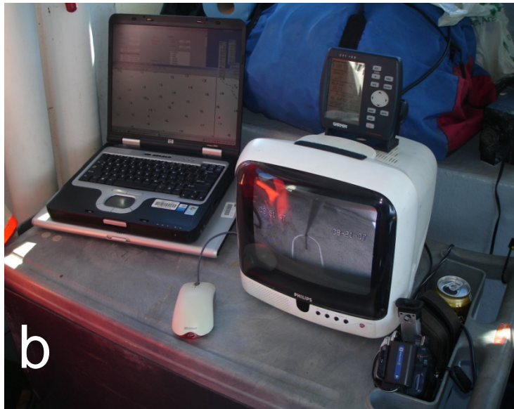
Figure 2. URCHIN camera system. (a) in between transects on deck. Low light black and white camera is at apex of tripod, looking forward; dual lasers are mounted at rear. Light (seldom used) is on left rear leg. Temperature recorder is strapped to same leg. (b) On-deck survey monitoring and data recording systems. Shown is laptop running geographical information system software, and a custom software program for time- and geo-referenced logging of discrete "events" (e.g. lobster encounter) and "classes" of habitat types (start and end points on the survey for each habitat class). GPS shown above TV monitor, with video camera for recording underwater video shown alongside. (c) Deploying URCHIN over the side of a lobster fishing boat
