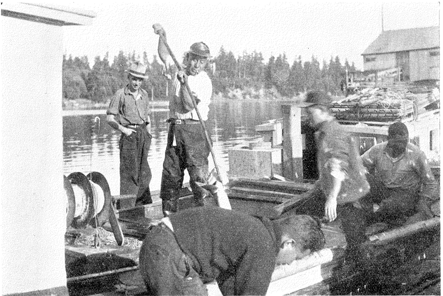
FIGURE 10. Type of boat used by Japanese in ling cod fishing in British Columbia. Note live well and jig with lines wound on drums to left of picture.
