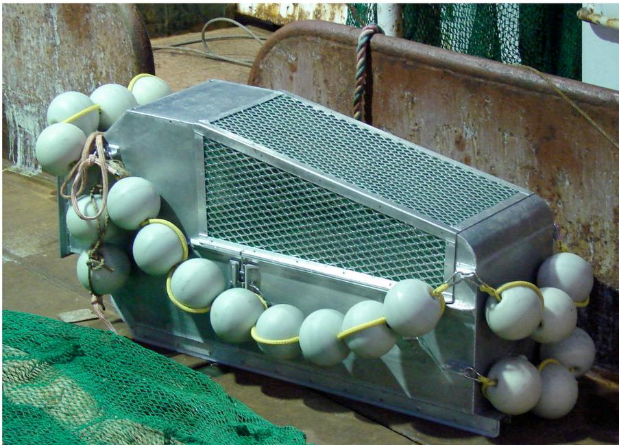
**Figure II-4 : “Aquarium” codend ready for attachment to net, showing array of trawl floats used during the 2008 survey. For the subsequent surveys, only minor modifications were made to the arrangement of floats.**
