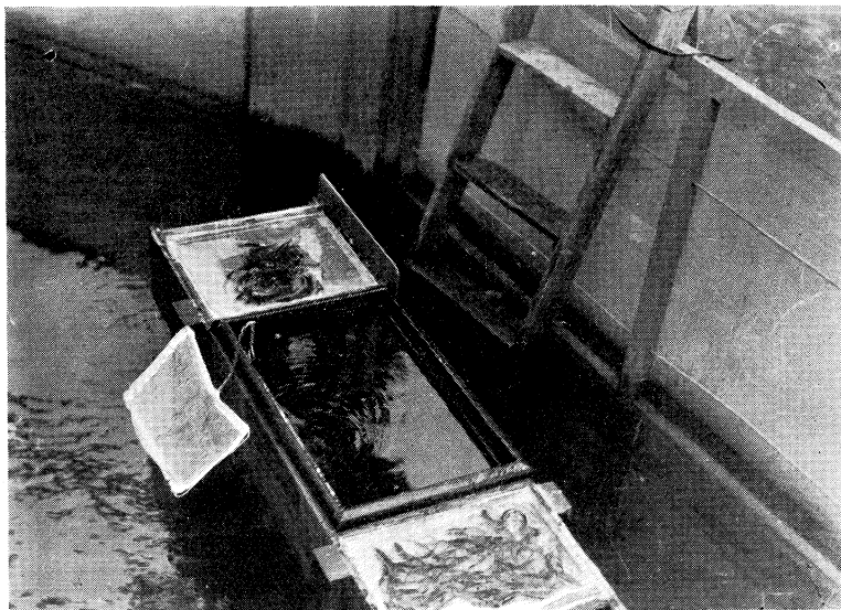
FIGURE 7. The apparatus used in counting seaward migrants. Placed right in the retaining pen it consists of a wooden trough, waist-high, with compartments at each end, covered by cloth screening, into which the fish are dipped, and a central portion built to hold a wire-screen hatchery basket into which the migrants are counted. The central basket is movable and when filled can be removed and emptied over the side of the pen, thus returning the fish to the creek to continue their seaward journey. The water can be drained off and replenished at any time. Four counters can work comfortably at such apparatus.
