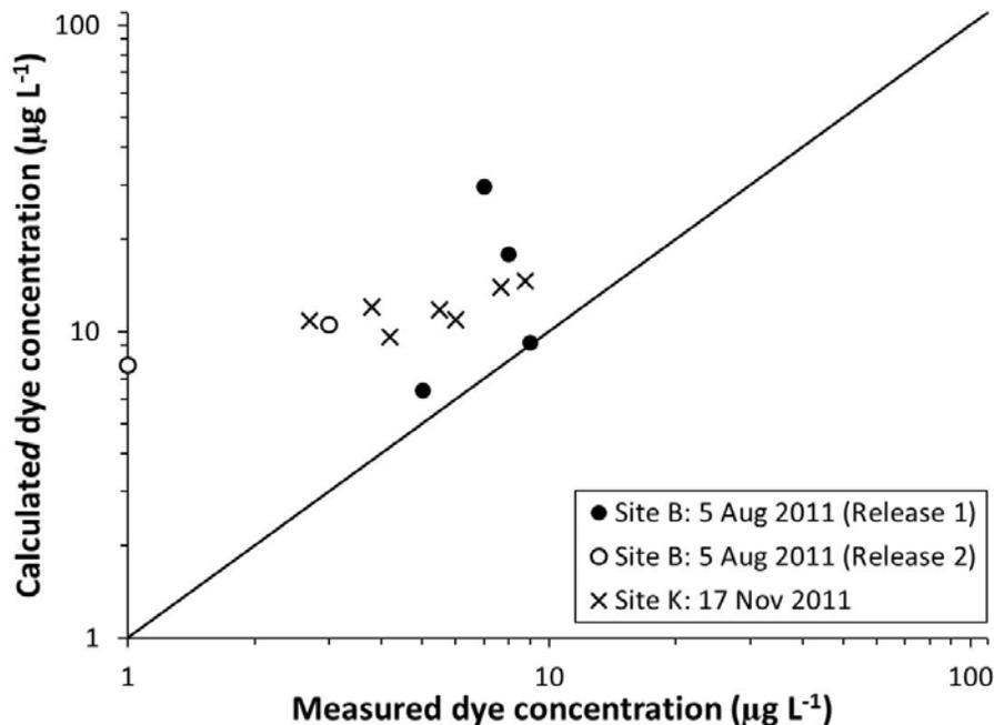
Figure 6: Comparison of measured and predicted dye concentrations in dye plumes resulting from well-boat treatments.
