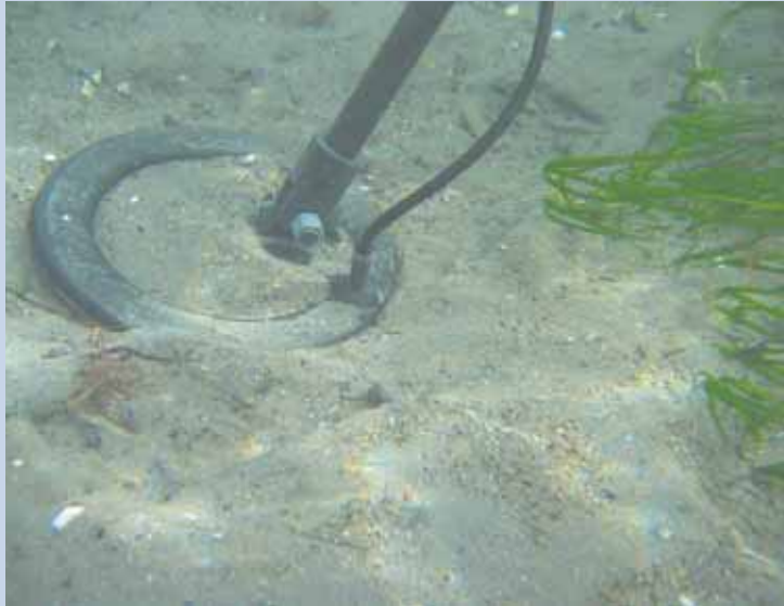
Metal detector used to locate tagged clams in the Malbaie barachois in the Gaspé Peninsula.
