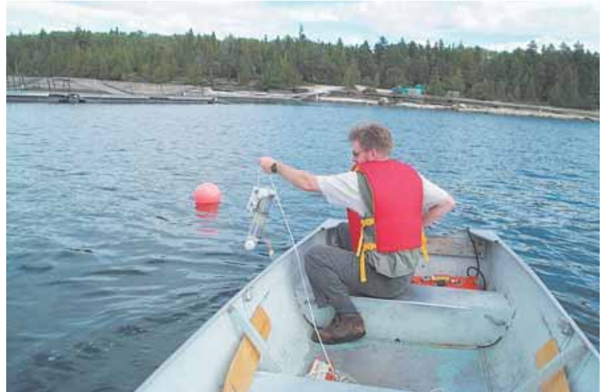
Post Doc Gregor Reid is collecting water samples adjacent to a commercial farm site to monitor diel fluctuations in dissolved phosphorus levels.
