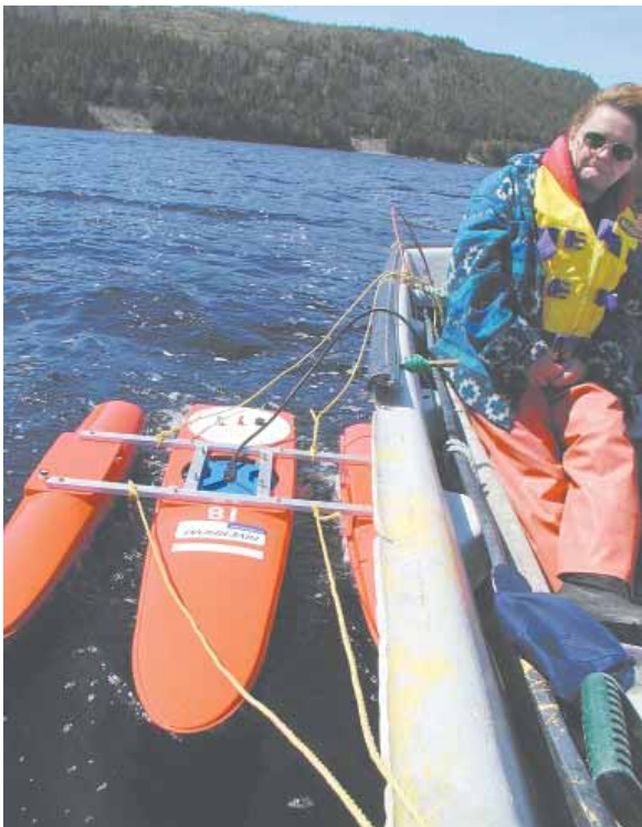
Environmental data collection with YSI Sonde profiler deployed by Sean Macneill Badger Bay Mussel Farms and Sharon Kenny DFO.
