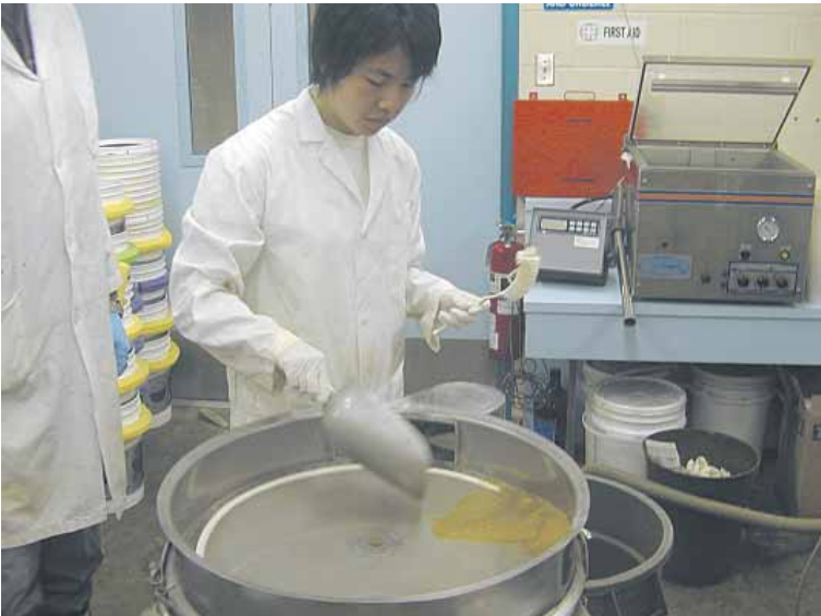
Susie Huang (M.Sc. Student, UBC) showing separation of crumbled pelleted feed into different fractions for fish of different sizes.
