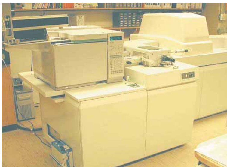
Analytical equipment at the DFO Institute of Ocean Sciences used for measurement of organohalogen compounds.
