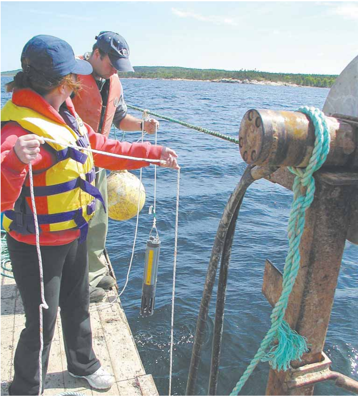
Riverboat flotation for acoustic Doppler profiler collecting current data at mussel aquaculture site with DFO Aquaculture technician Sharon Kenny.
