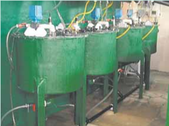
Computer-controlled, and automated, tank respirometry system used to measure the cost of digestion in groups of juvenile Atlantic cod and haddock.
