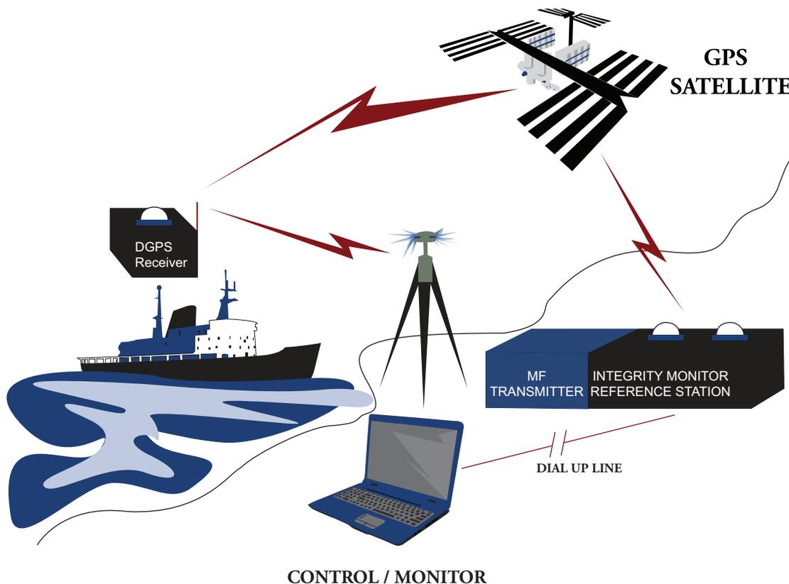
A reference station is established at a known geodetic location and position information received from the GPS satellites is compared to this known geodetic location. Based on this information, differential corrections are generated and broadcast to the user via Marine MF radiobeacons.
