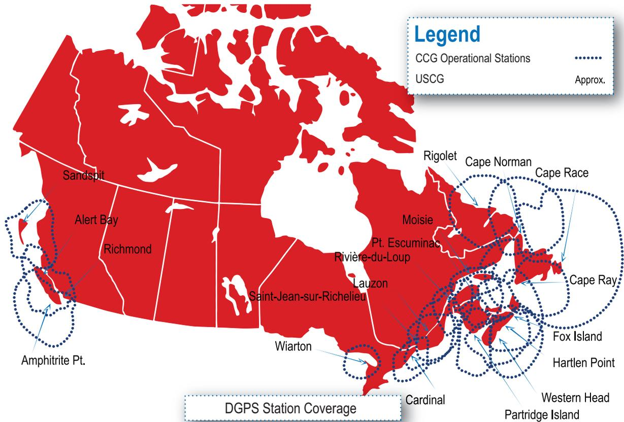
A method of obtaining greater accuracy from GPS is through a technique called Differential GPS (DGPS). This technique corrects the inherent inaccuracies of the GPS signal by comparing the position calculated by GPS to a known geographic position.
