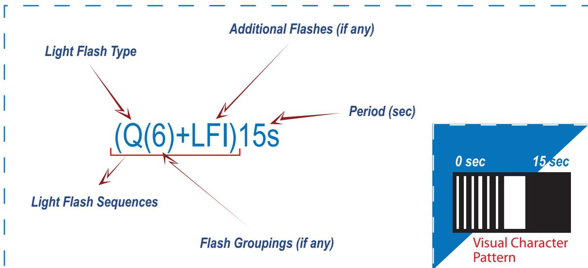
In all cases, the first letter(s) in the light flash character gives reference to the general light flash type or classification. This classification is based on the duration of illumination in relation to eclipse (darkness) for each light flash. In the example on page 20, the letter “Q” indicates that the aid is equipped with a quick flashing light; a quick flashing light being one which flashes at a rate of one flash per second.
